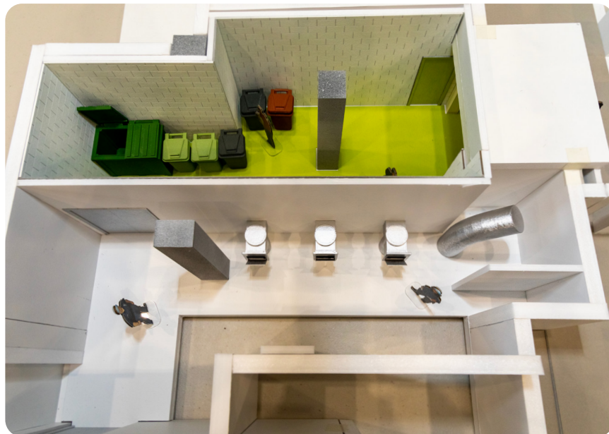
Physical model showing resident and staff facing areas of the recycling room. Resident area (with green floor) shows hopper doors for system and bins for other materials.
