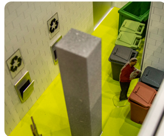
Physical model showing resident and staff facing areas of the recycling room. Resident area (with green floor) shows hopper doors for system and bins for other materials.
