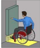
Toe space (9" high min.): Max. depth 6"
