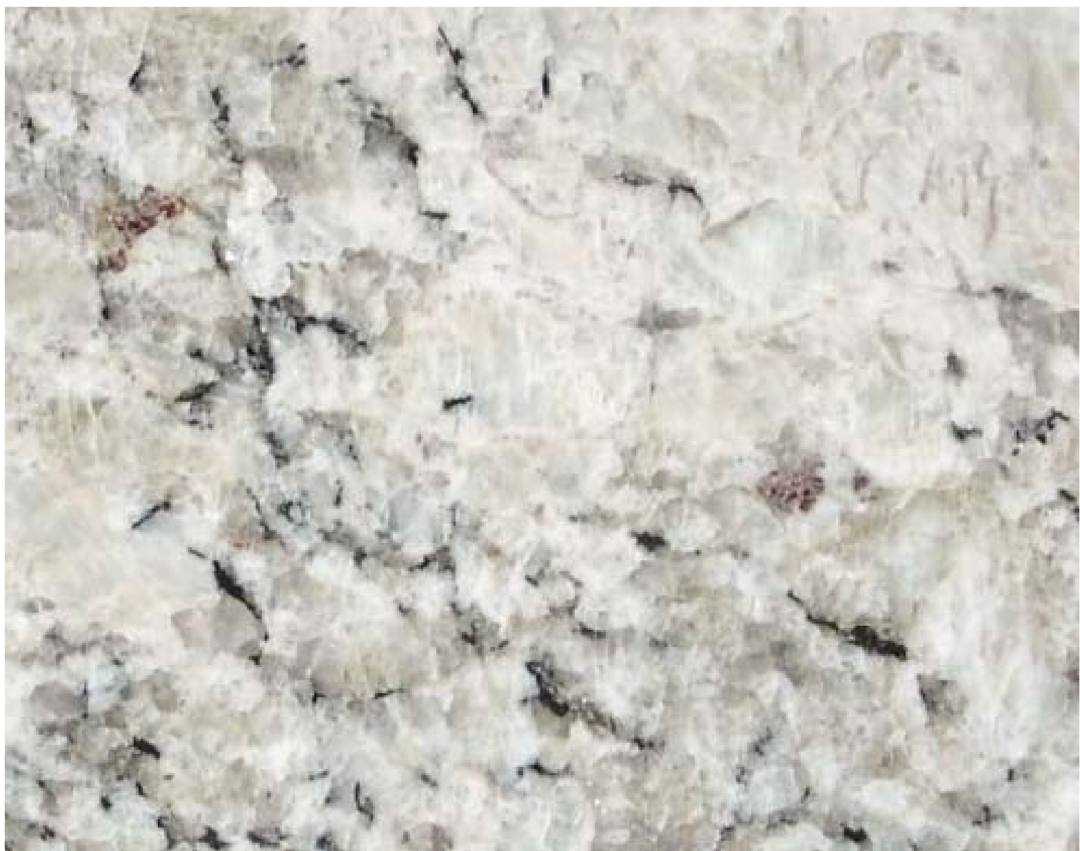
CUSTOM GRANITE SEATWALL SLABS AND COFFEE TABLE COLOR : SALT AND PEPPER FINISH : HONED
