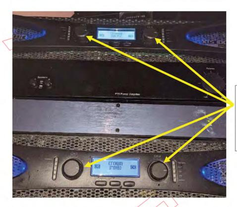
The four volume controls on the two stereo amplifiers were previously set to approximately 75%. Now they are now set to maximum so they cannot be turned up higher to override the limiter settings.
