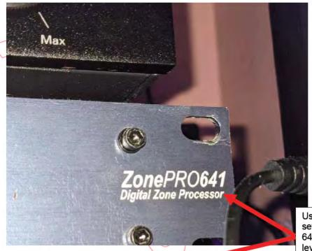
Using a computer to access the settings on the DBX Zone Pro 641, I properly set the limiter levels.
