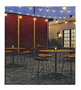
Sound Seal Sound Curtain Panels will be installed on free-stand walls built out to avoid fastening to the funeral home building facade.
