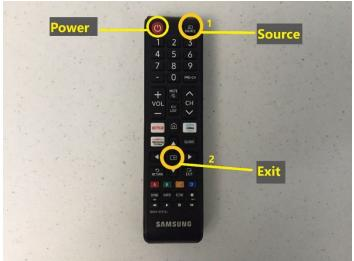
7. If the TV menu is on the screen use the 'exit' button on the remote to clear it. The exit button's location on the remote control is shown in the image below.
