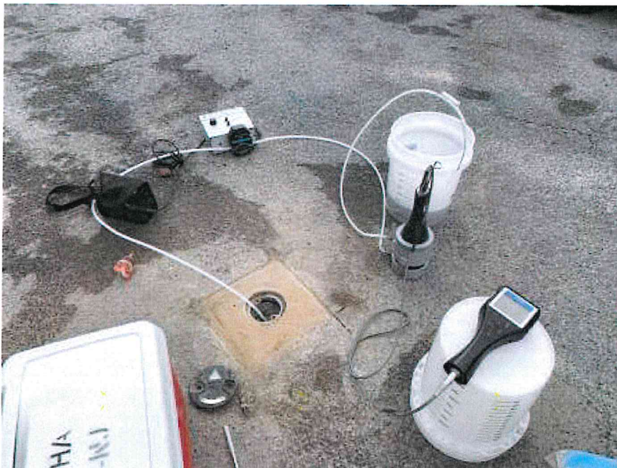
Photo 4: Typical groundwater sampling set up
