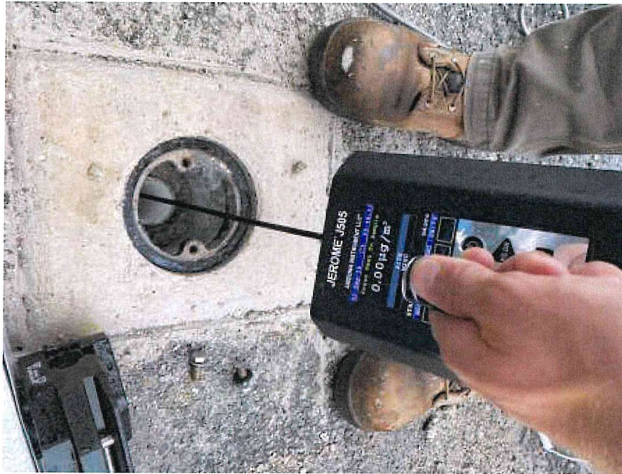
Photo 3: Jerome screening at monitoring well MW34
