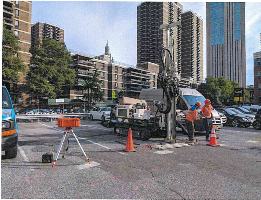
Photo 1: AARCO advancing soil boring SB20 in the northern part of the site (facing north)
