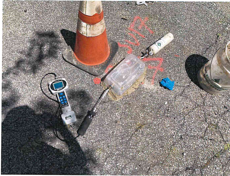
Photo 3: View of helium tracer test at SV-17
