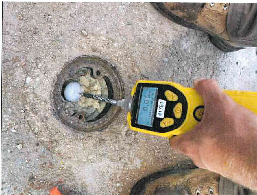
Photo 2: PID screening of monitoring well MW33
