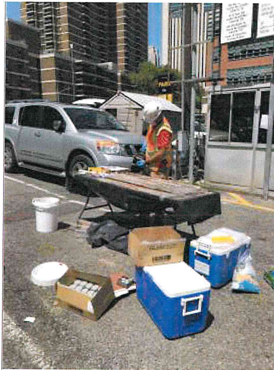
Photo 3: Langan collecting mercury vapor readings from a soil boring (facing northeast)
