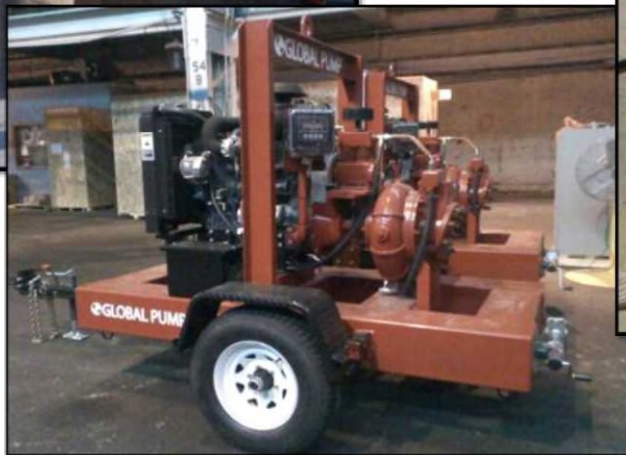
Mobile Diesel Flood Pumps
