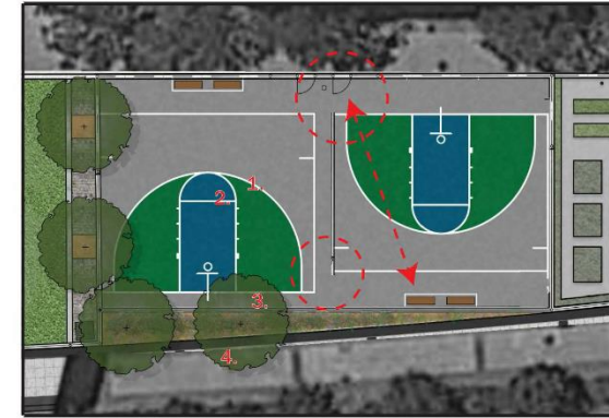
NORTHERN COURT ROTATED 180°, BENCHES MOVED TO EAST SIDE
