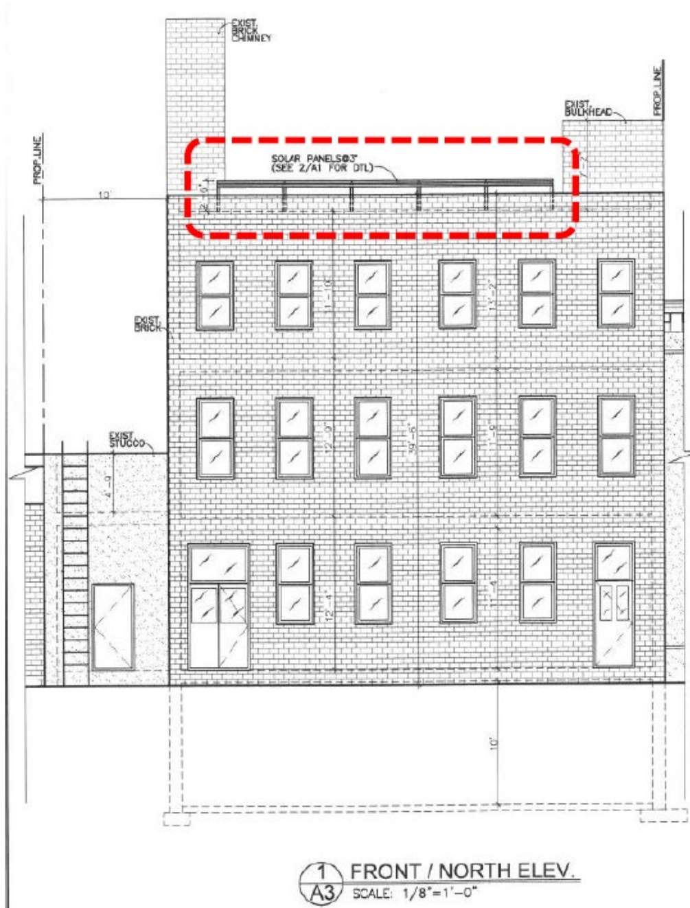
Figure 7: Solar panel installation "B" as positioned behind the front façade parapet.
