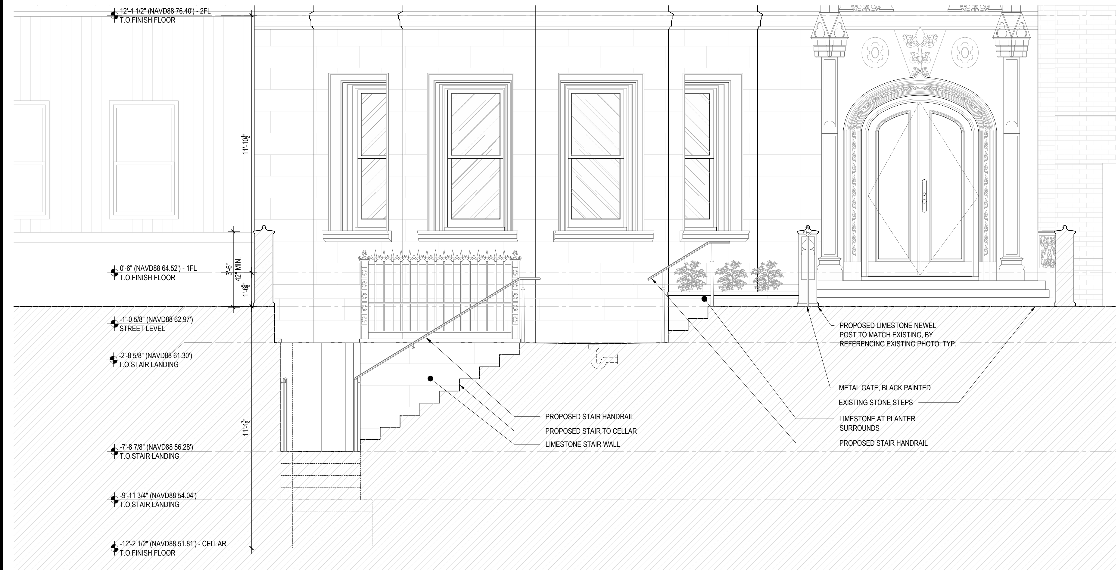
1 PROPOSED CELLAR STAIR SECTION SCALE: 3/8" = 1'-0"
