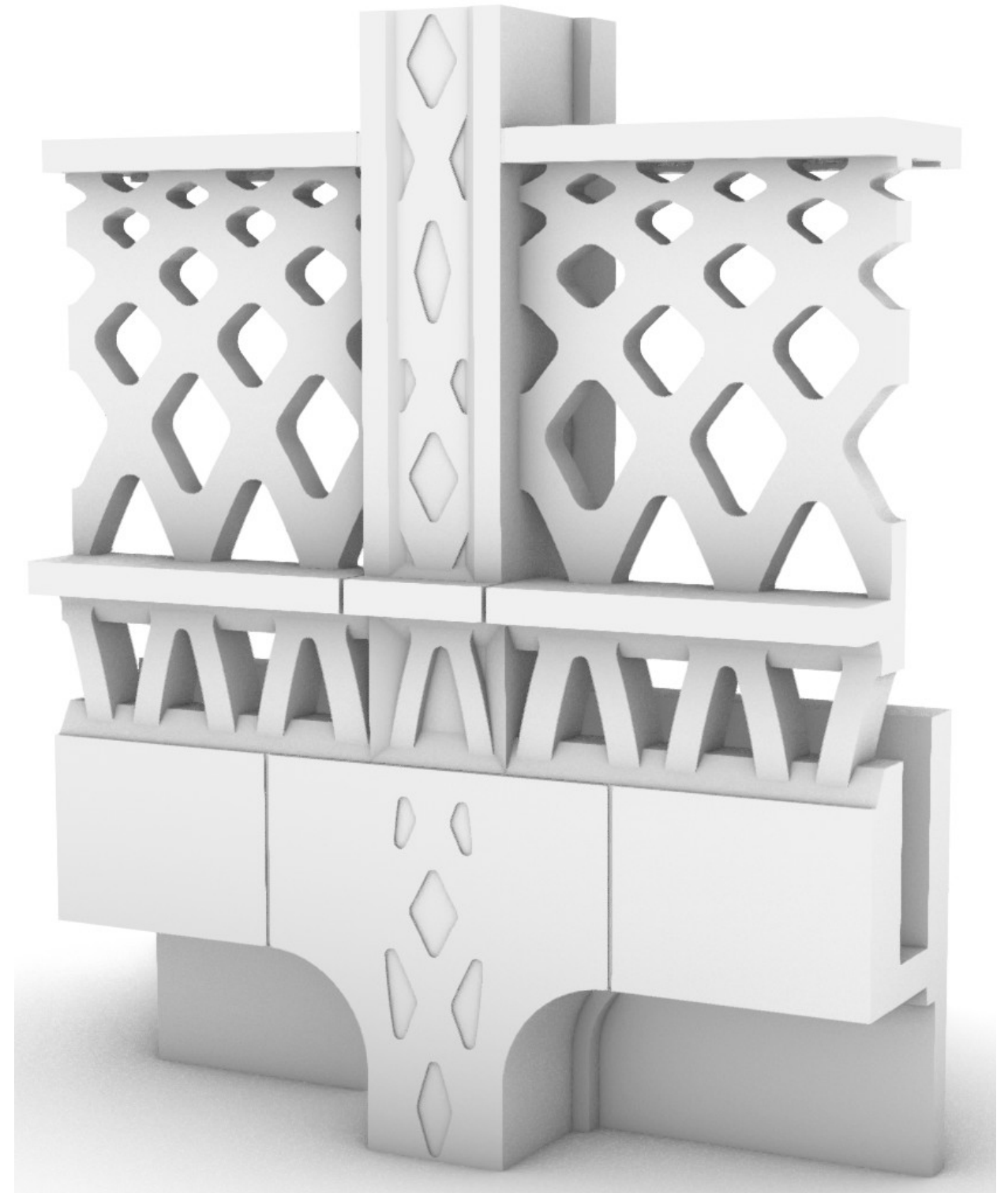
1:2 scale model of proposed facade design
