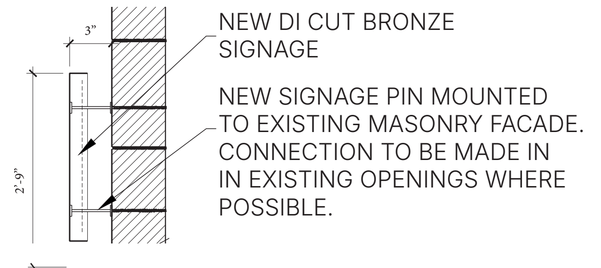
BRONZE PLAQUE SIGNAGE SECTION DETAIL
