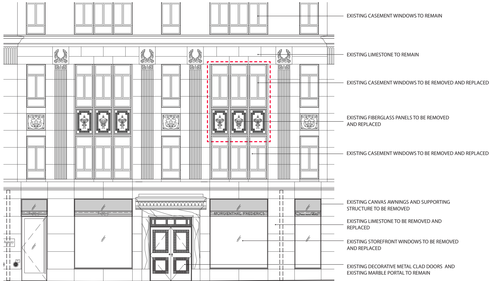
EXISTING ELEVATION AT BUILDING
