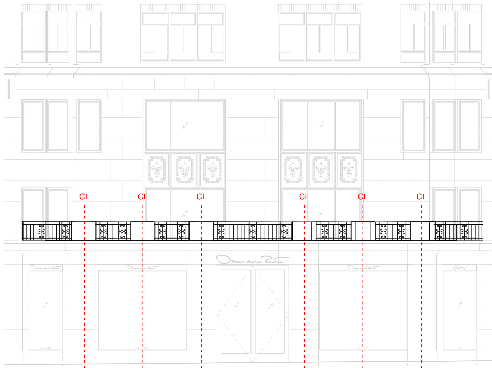
PROPOSED ELEVATION - RAILING AND BALUSTRADE
