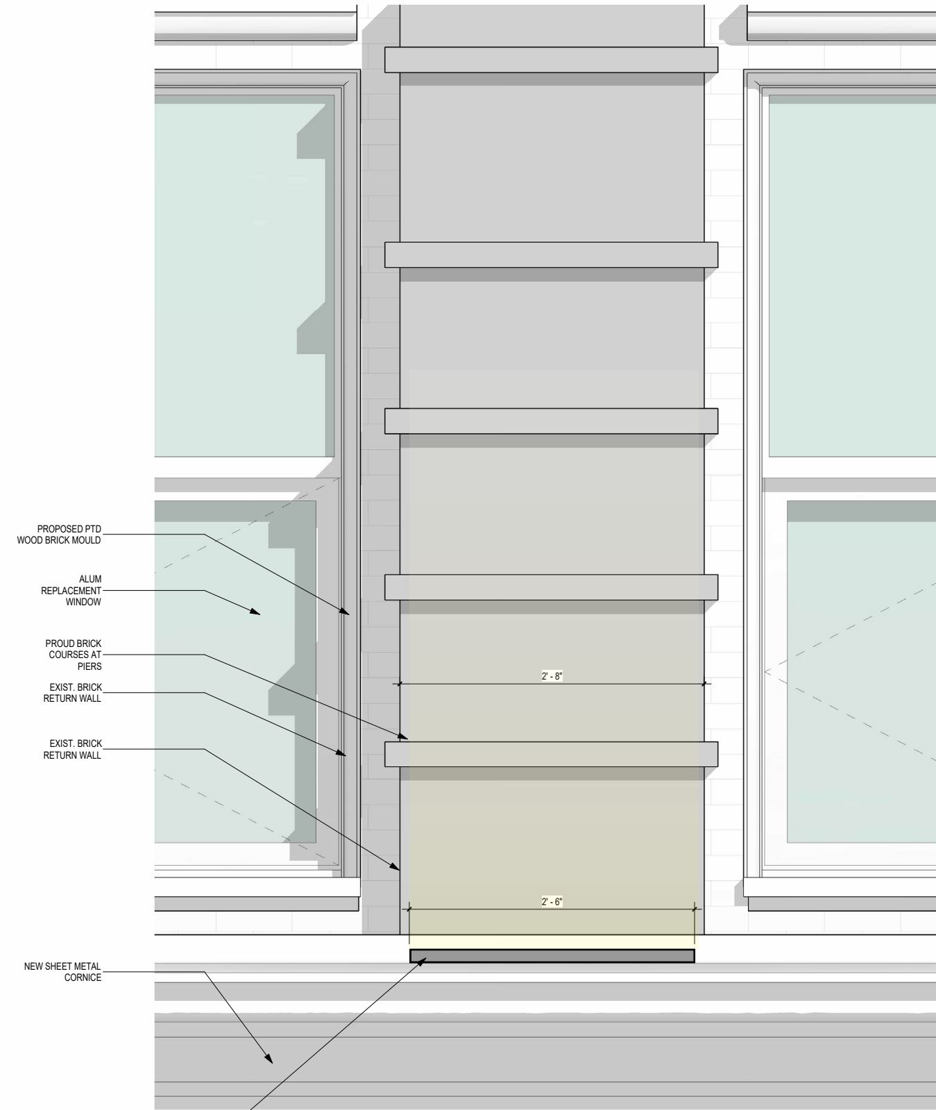
BRICK PIER ELEVATION
