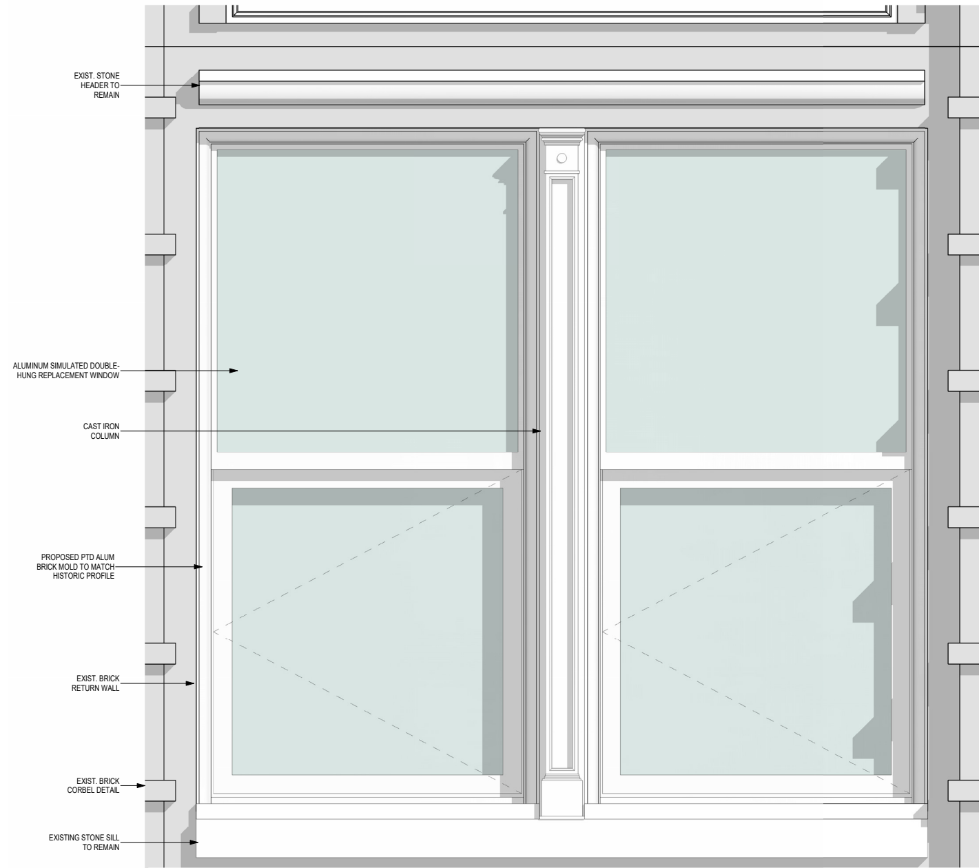
② PROPOSED SIMULATED DOUBLE-HUNG WINDOW 1 1/2" = 1'-0"
