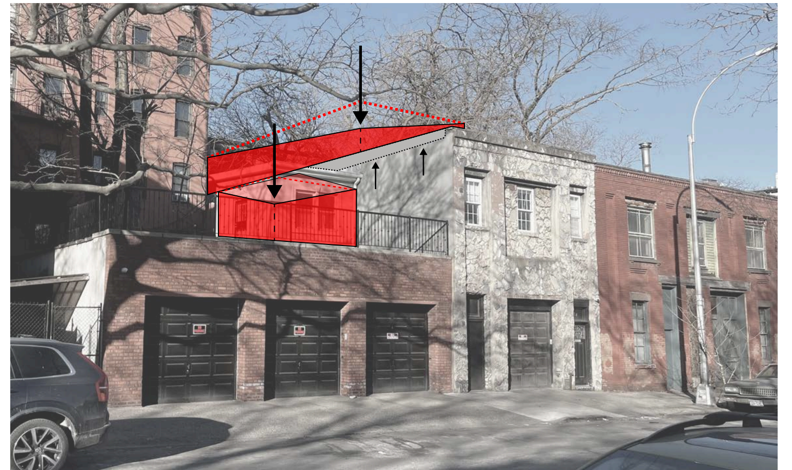
Massing of extension volumes with sloped roofs and raised parapet to minimize visibility
