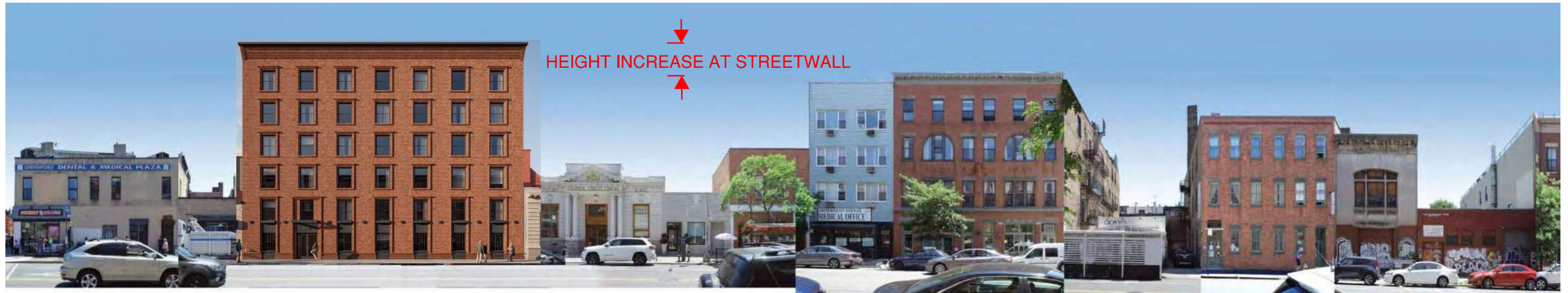
REVISED STREET ELEVATION : INCREASED STREETWALL - CORRUGATED HEIGHTS AT SOUTH SIDE OF GREENPOINT AVENUE
