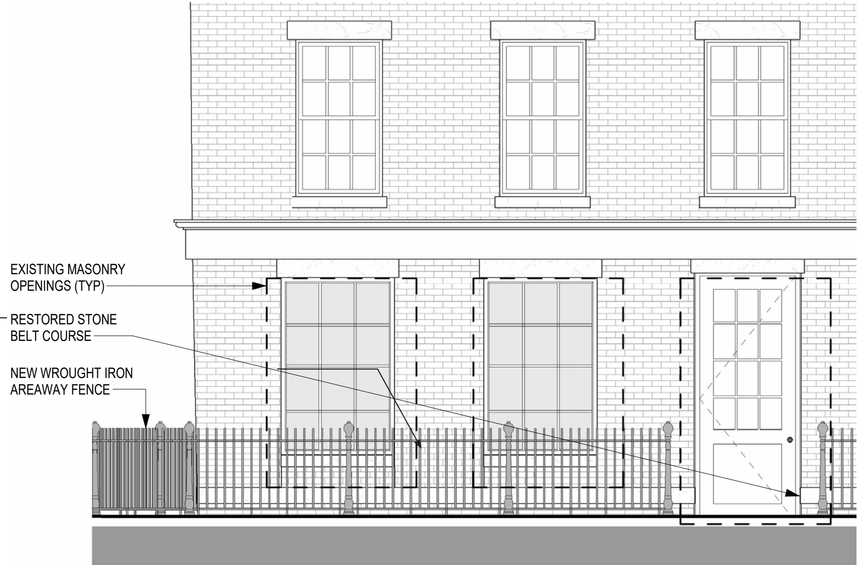
PROPOSED PARTIAL HUDSON ST ELEVATION
