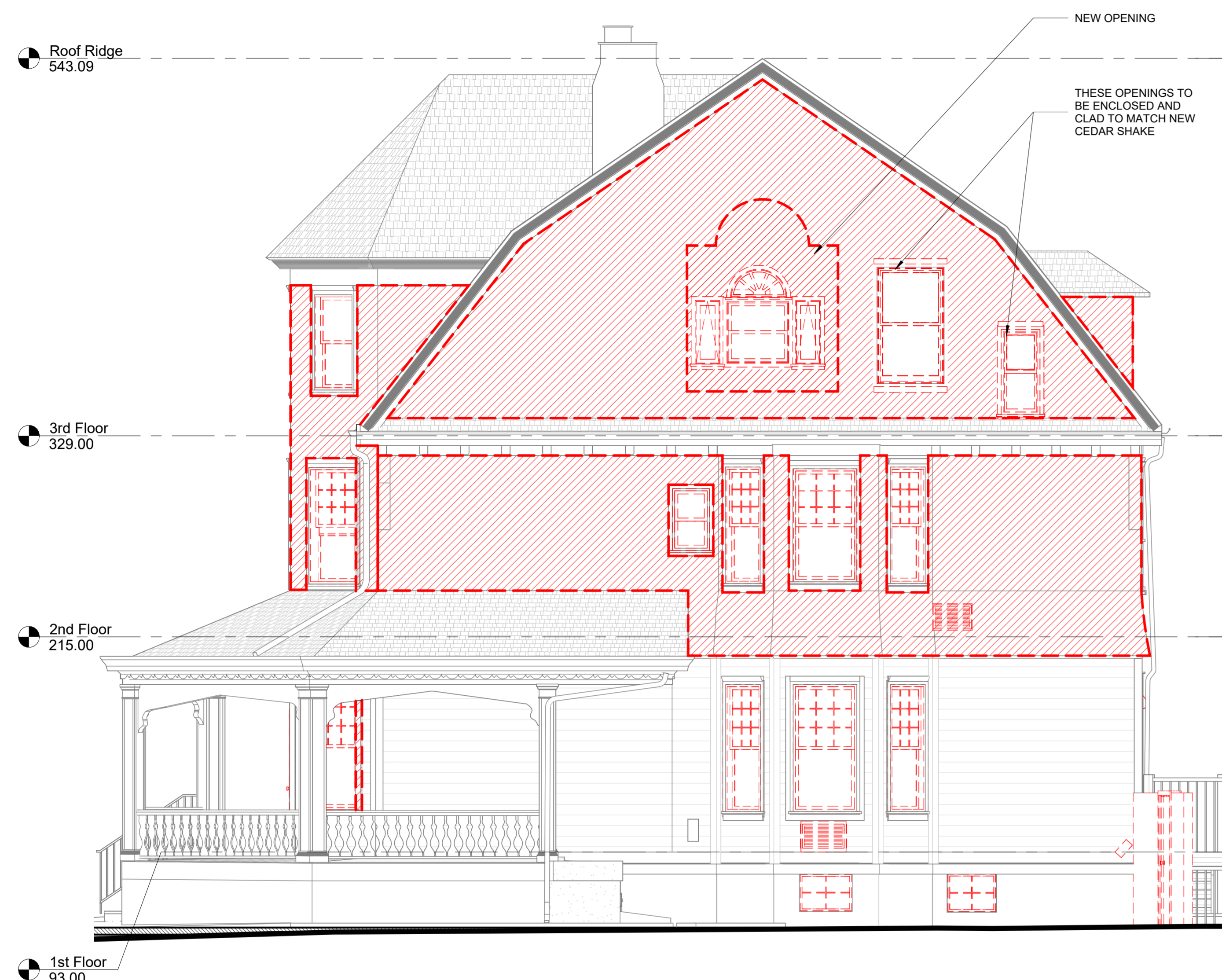
1 SOUTH ELEVATION - DEMO 1/4" = 1'-0"
