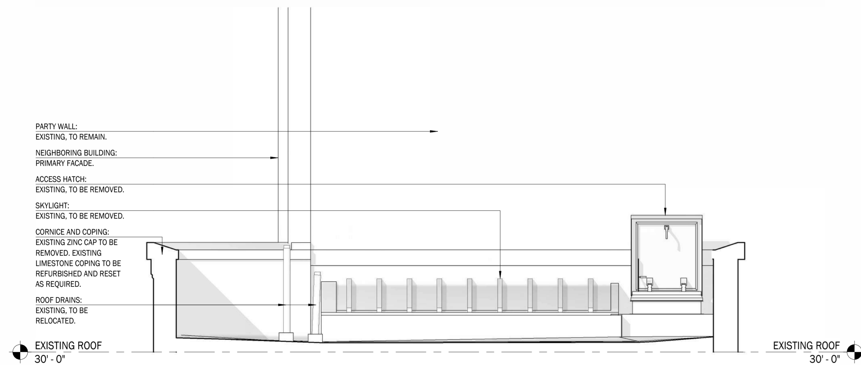
DRAWING 3 | EAST ELEVATION AT ROOF: EXISTING
