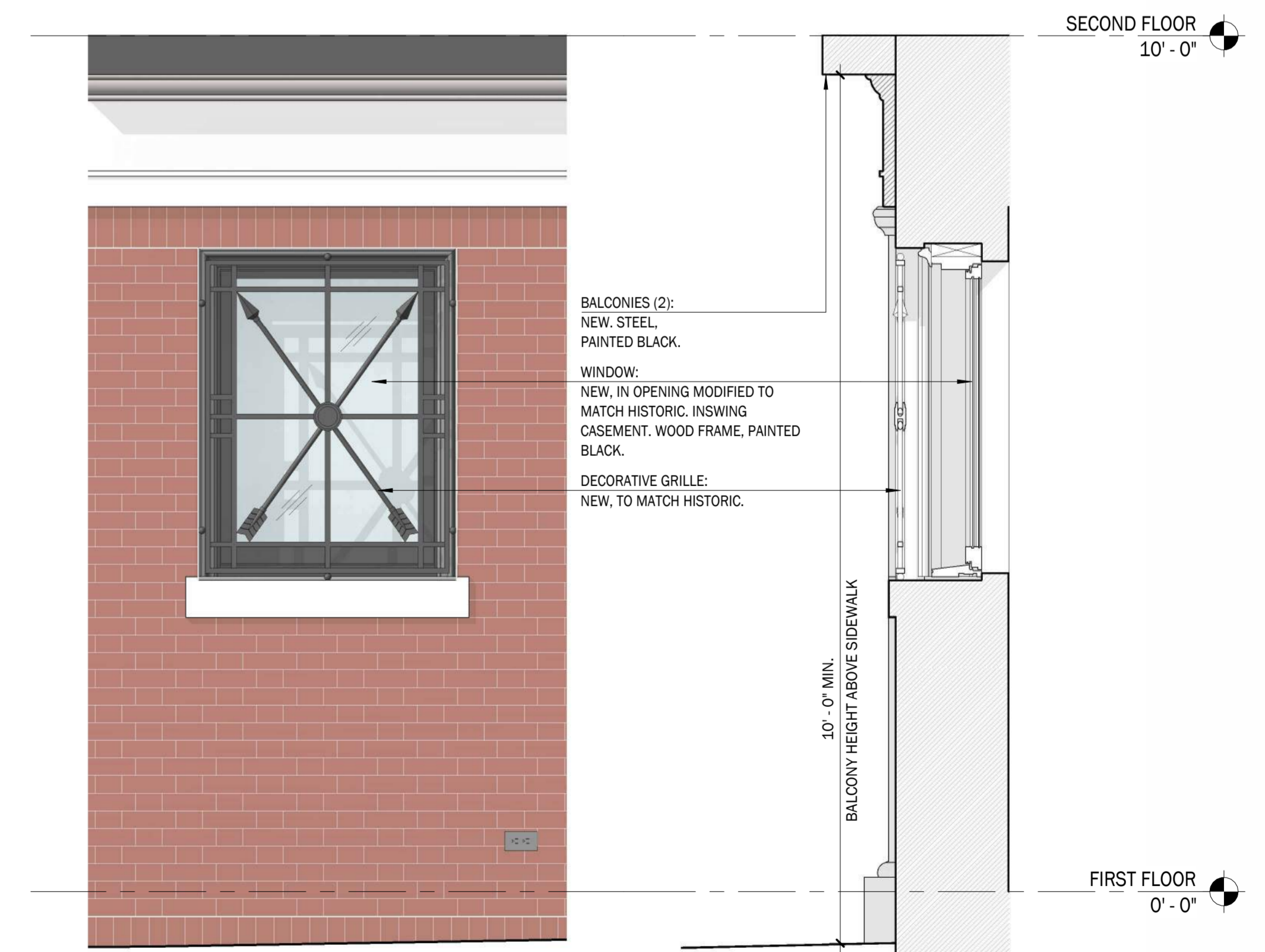
DRAWING 4A | ENLARGED ELEVATION: NEW WINDOW TO MATCH HISTORIC | 3/4" = 1'-0"
