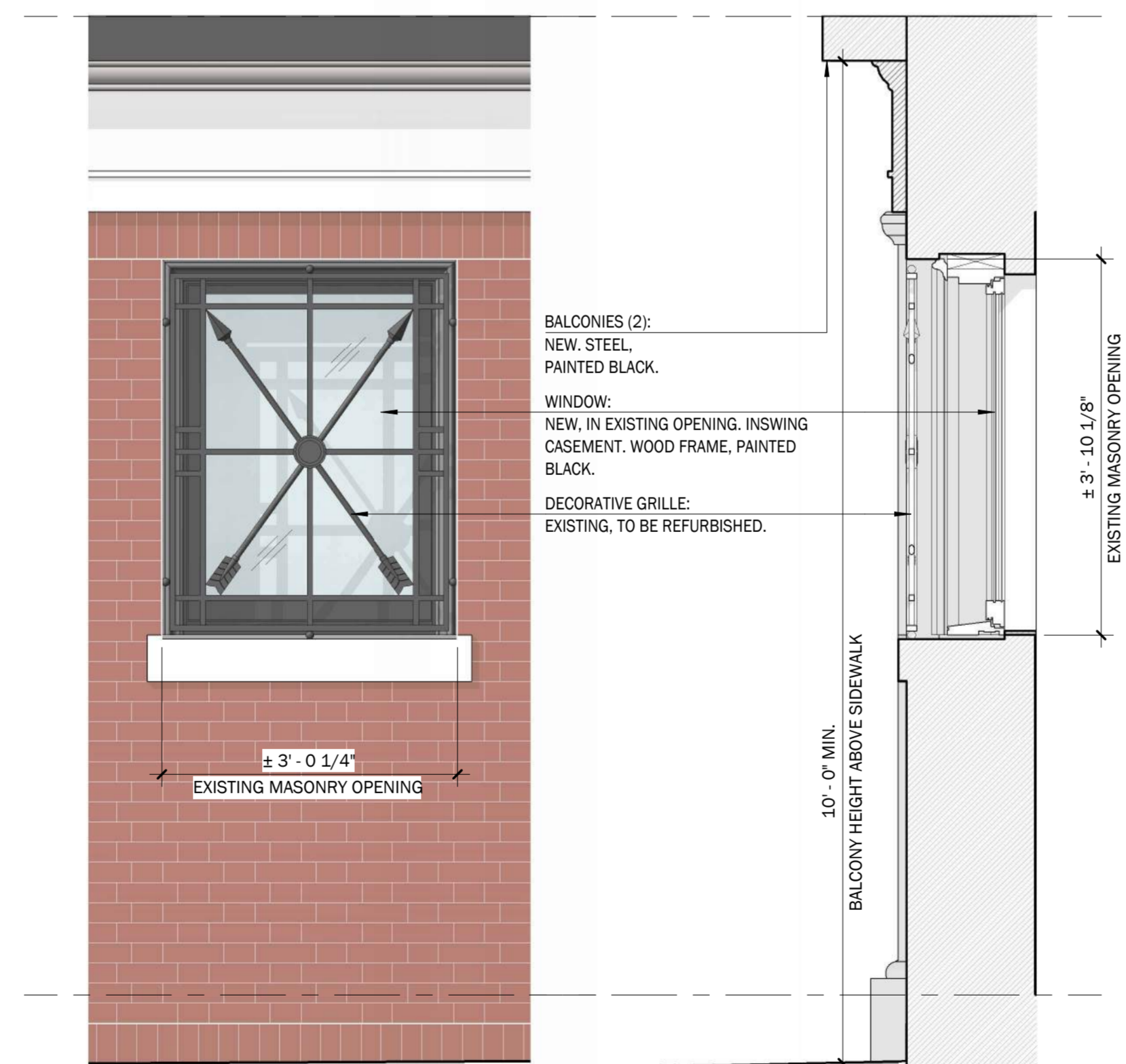
DRAWING 3A | ENLARGED ELEVATION: INSWING CASEMENT WINDOW | 3/4" = 1'-0"
