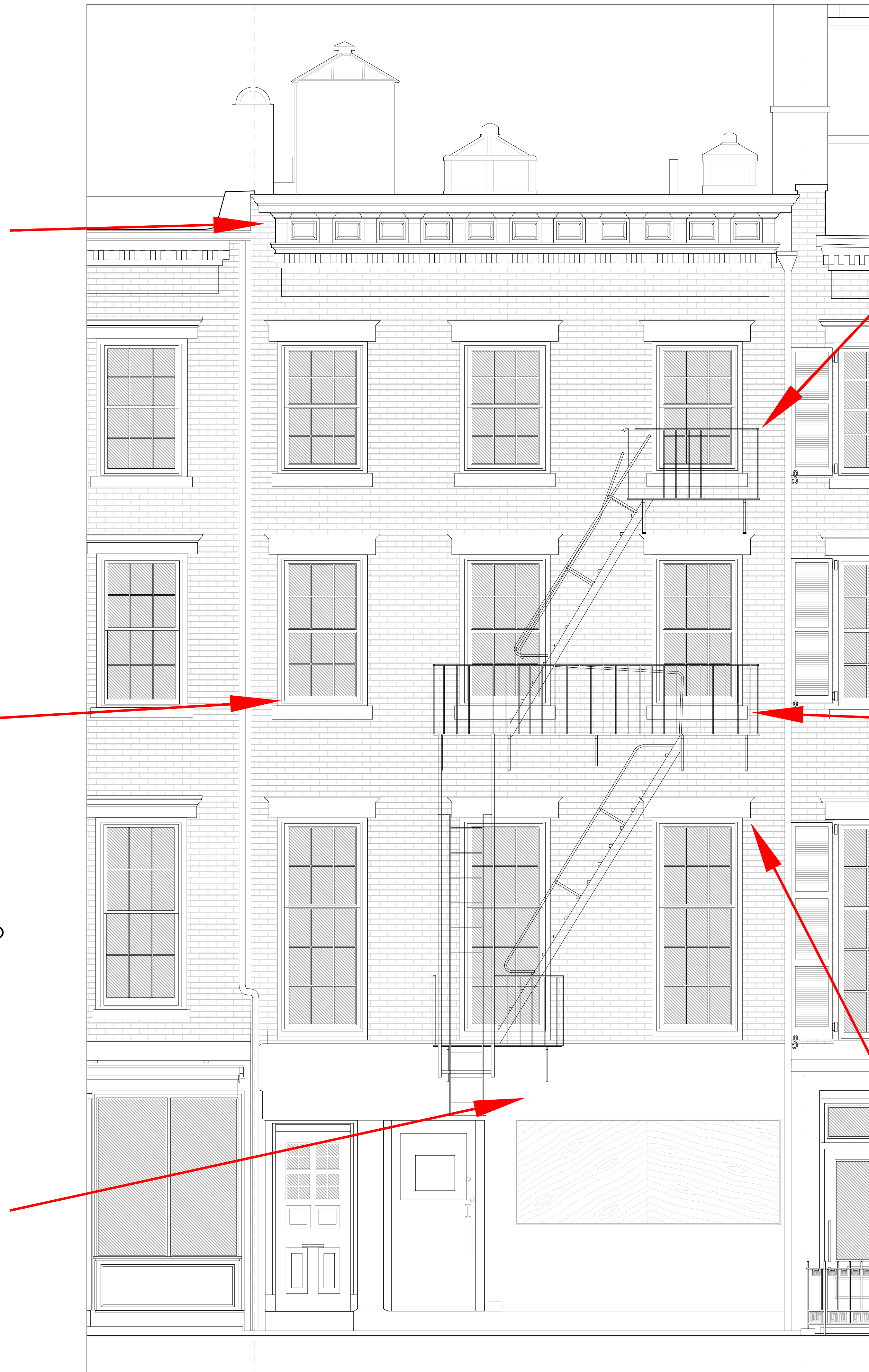
NON-ORIGINAL WINDOWS WITH NO BRICK MOULD OR CAULKING
