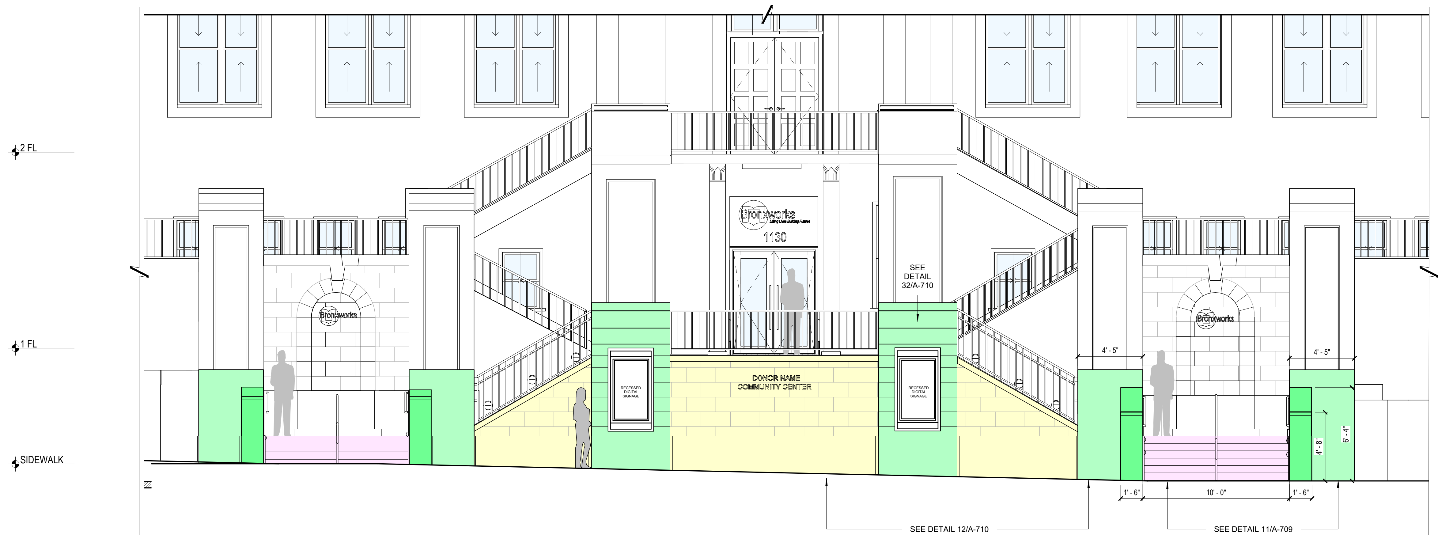
10 PROPOSED - WEST ELEVATION STEPS & ENTRANCE AREA (EXISTING STONE ELEMENTS NOT DRAWN) 1/4" = 1'-0"
