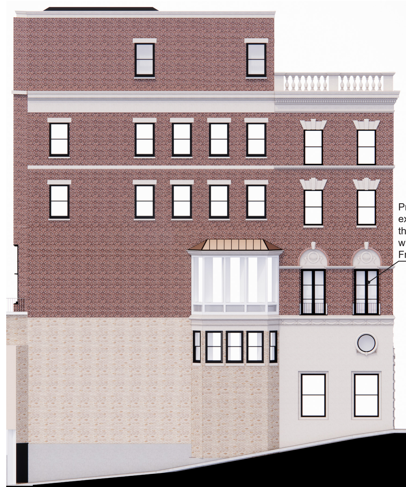
PROPOSED DESIGN - FRENCH DOORS ON 2ND FLOOR BALCONY
