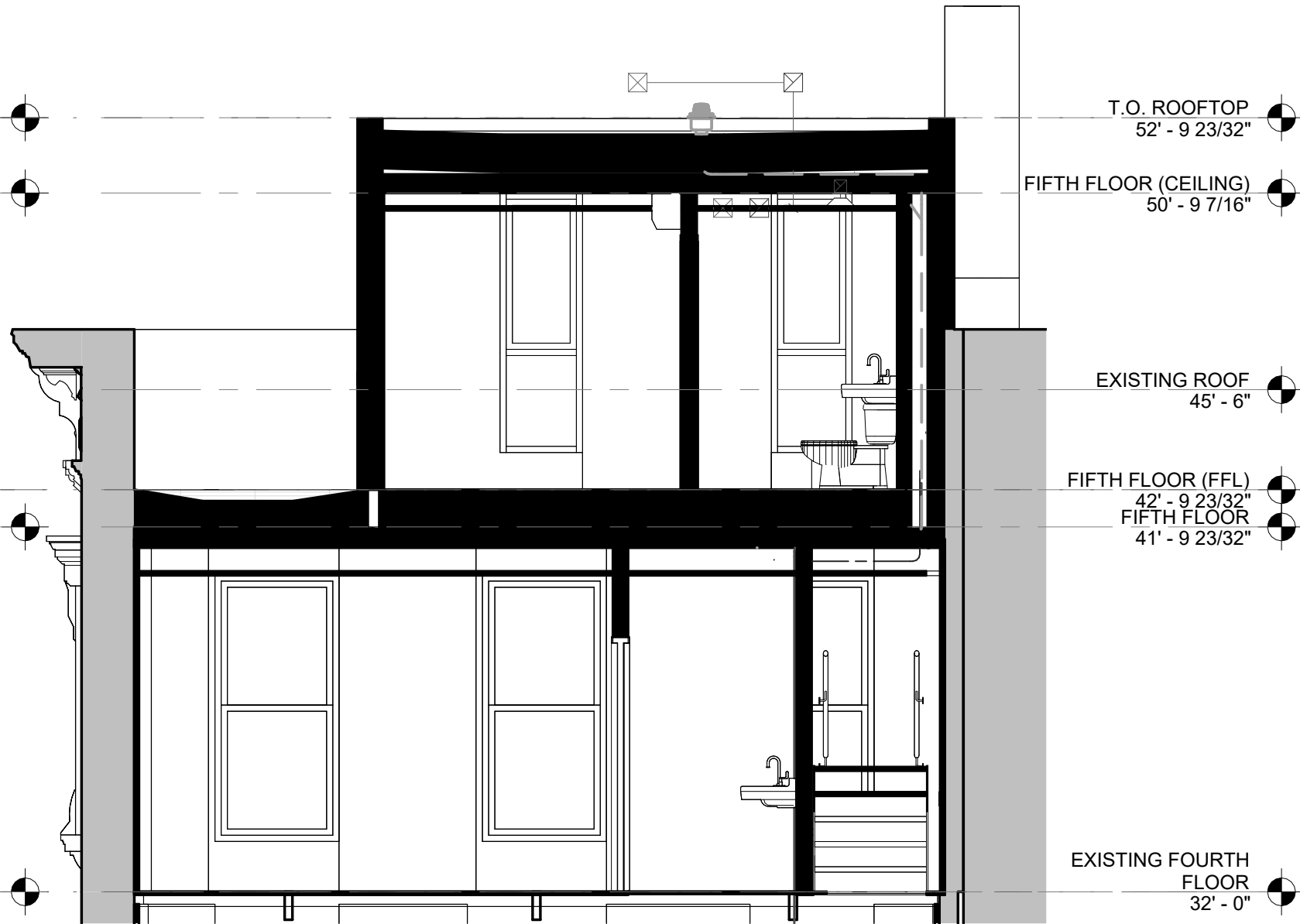
2 SECTION - ROOFTOP ADDITION (E-W SECTION #2) LPC-14 1/4" = 1'-0"
