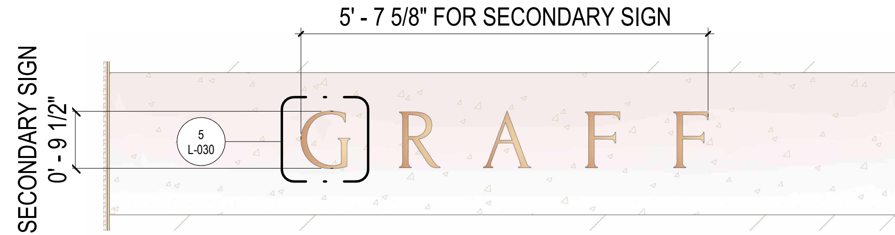
4 ENLARGED SECONDARY SIGNAGE 3/4" = 1'-0"
