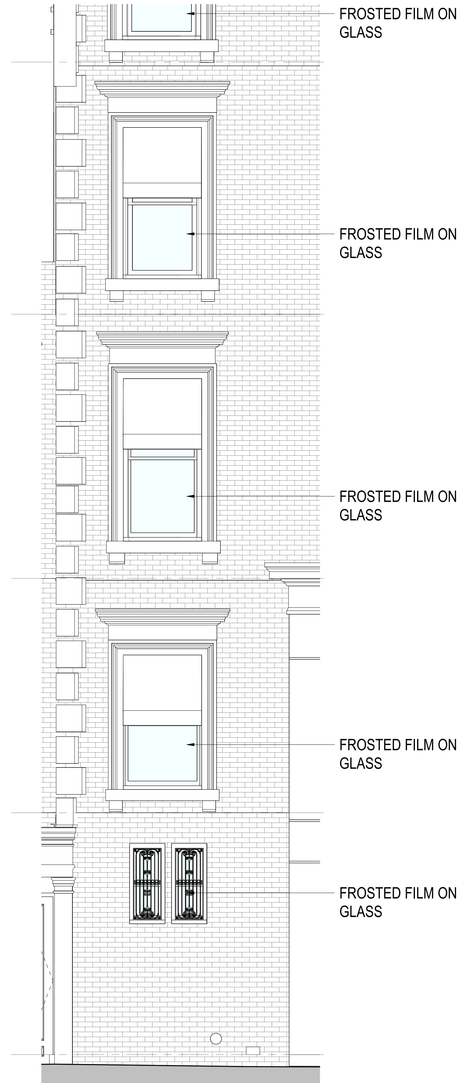
5 ELEVATION WINDOWS STAIR B 3/8" = 1'-0"
