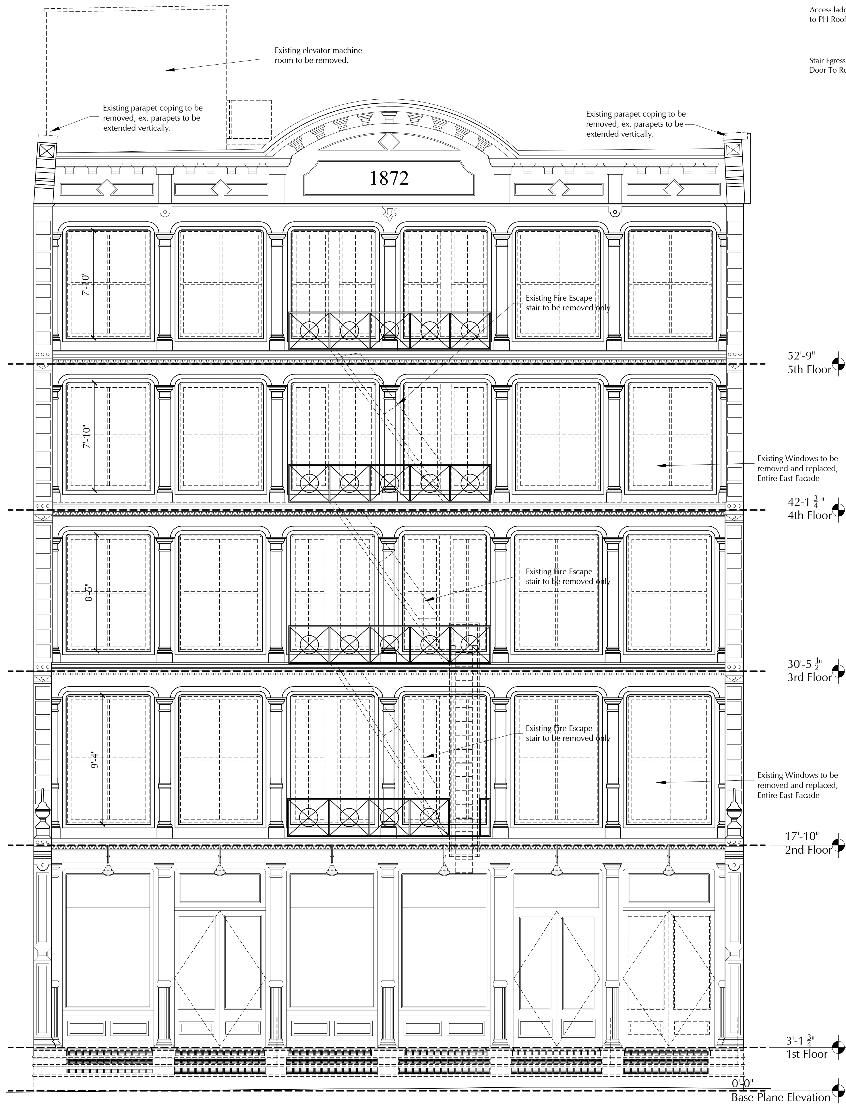
① Existing Front (East) Elevation 1/4" = 1'-0"
