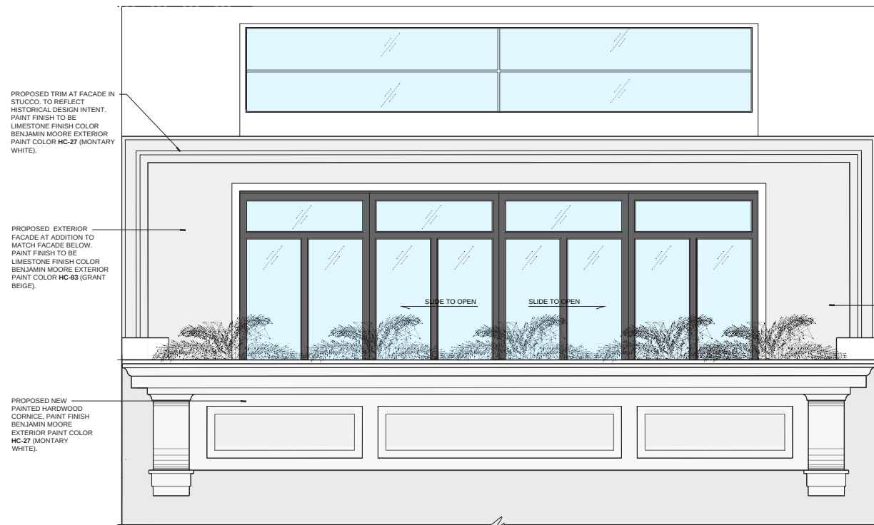
01 PROPOSED FRONT FACADE AT NEW ADDITION
