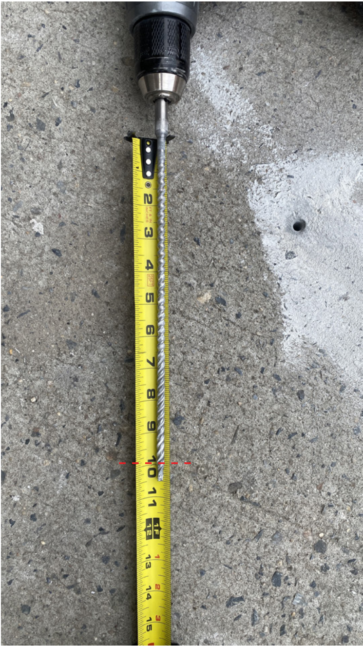
DEPTH PROBE No. 2 = 10" EAST VAULT ON METAL DECK
