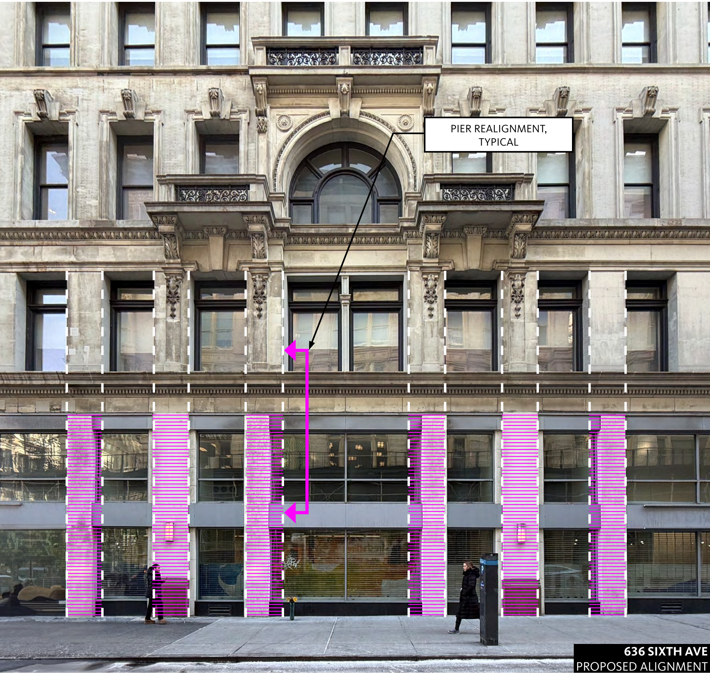
REFERENCING HISTORICAL INFLUENCE BY REALIGNING FLOOR 01 PIER PROPORTIONS TO UPPER LEVELS, INFILLING WITH FULL-HEIGHT STOREFRONT
