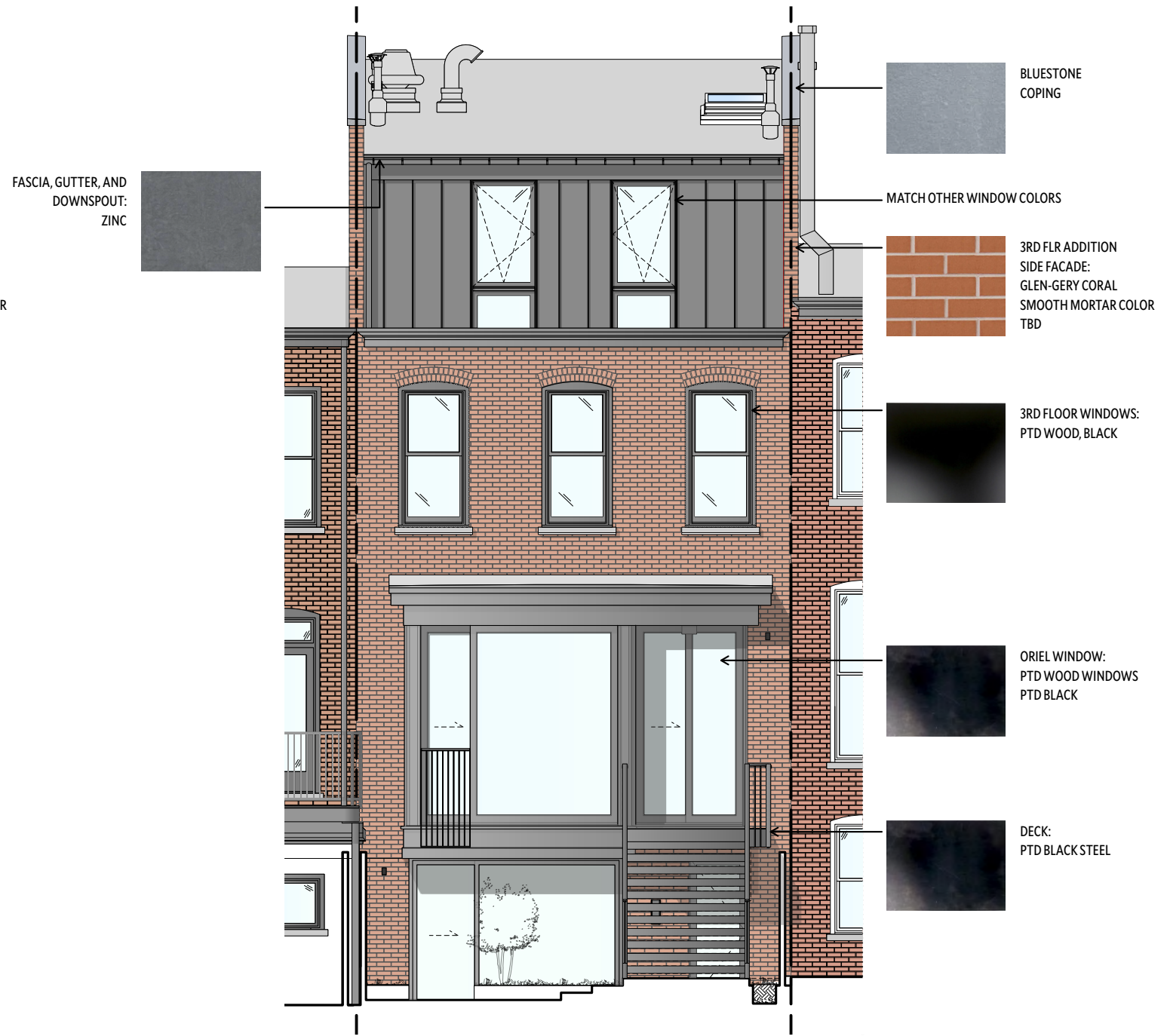
PROPOSED (08.12.2025) REAR ELEVATION WITH MATERIALS
