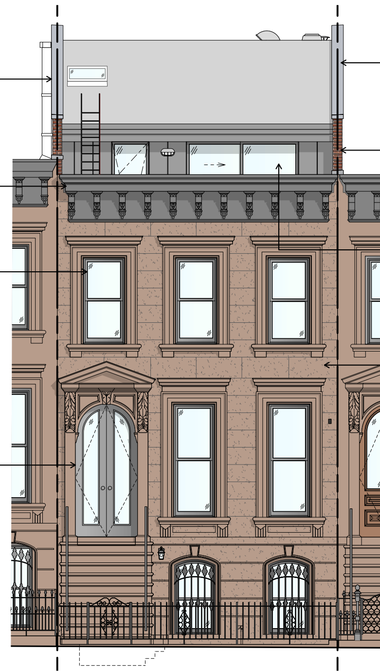
PROPOSED (08.12.2025) STREET ELEVATION WITH MATERIALS
