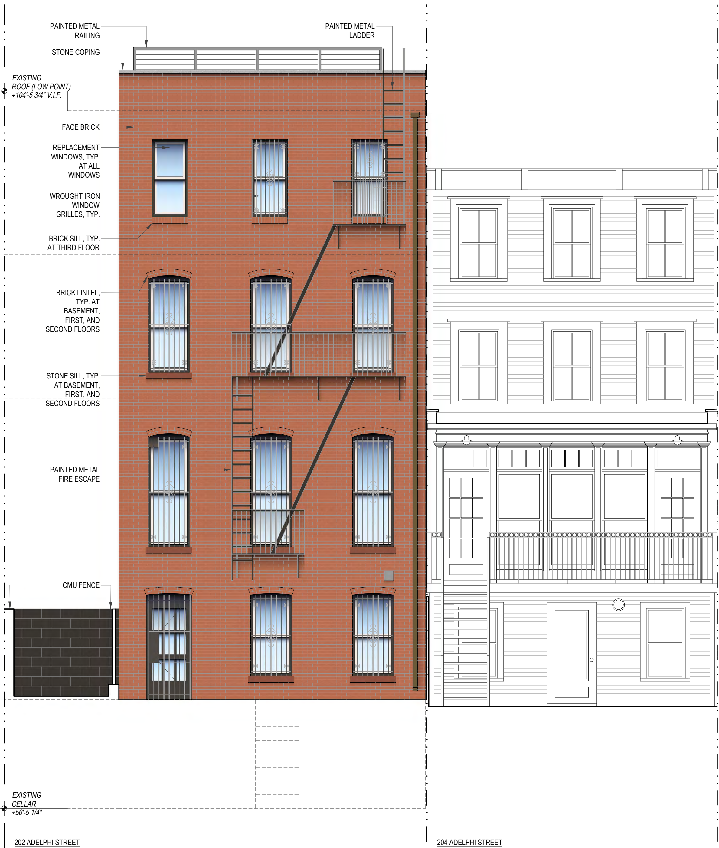
01 EXISTING ELEVATION: WEST (REAR) SCALE: 1/4" = 1'-0"
