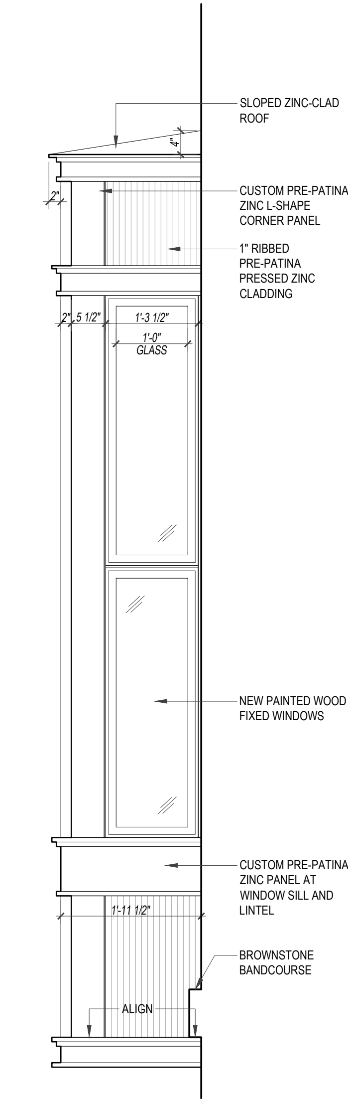
02 ORIEL WINDOW WEST ELEVATION SCALE: 3/4" = 1'-0"
