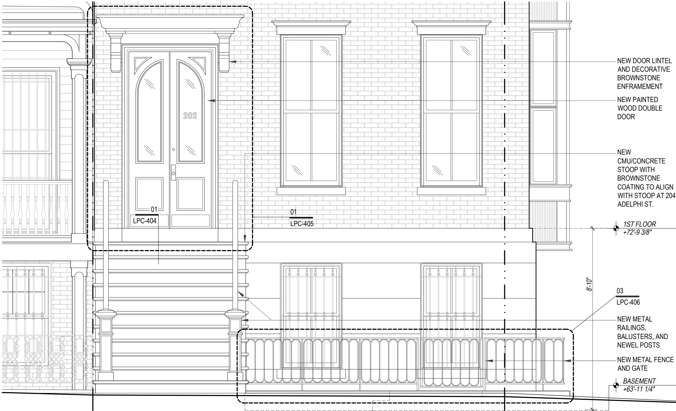
04 PROPOSED STOOP ELEVATION SCALE: 3/8" = 1'-0"
