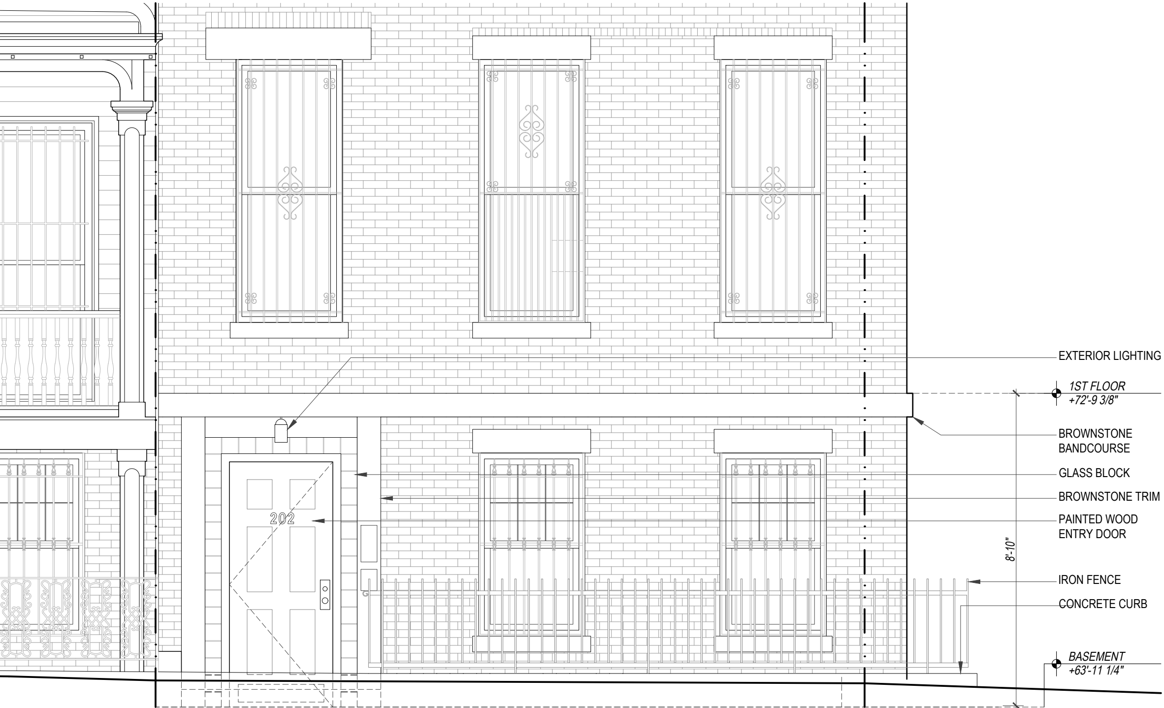
03 EXISTING AREAWAY ELEVATION SCALE: 3/8" = 1'-0"
