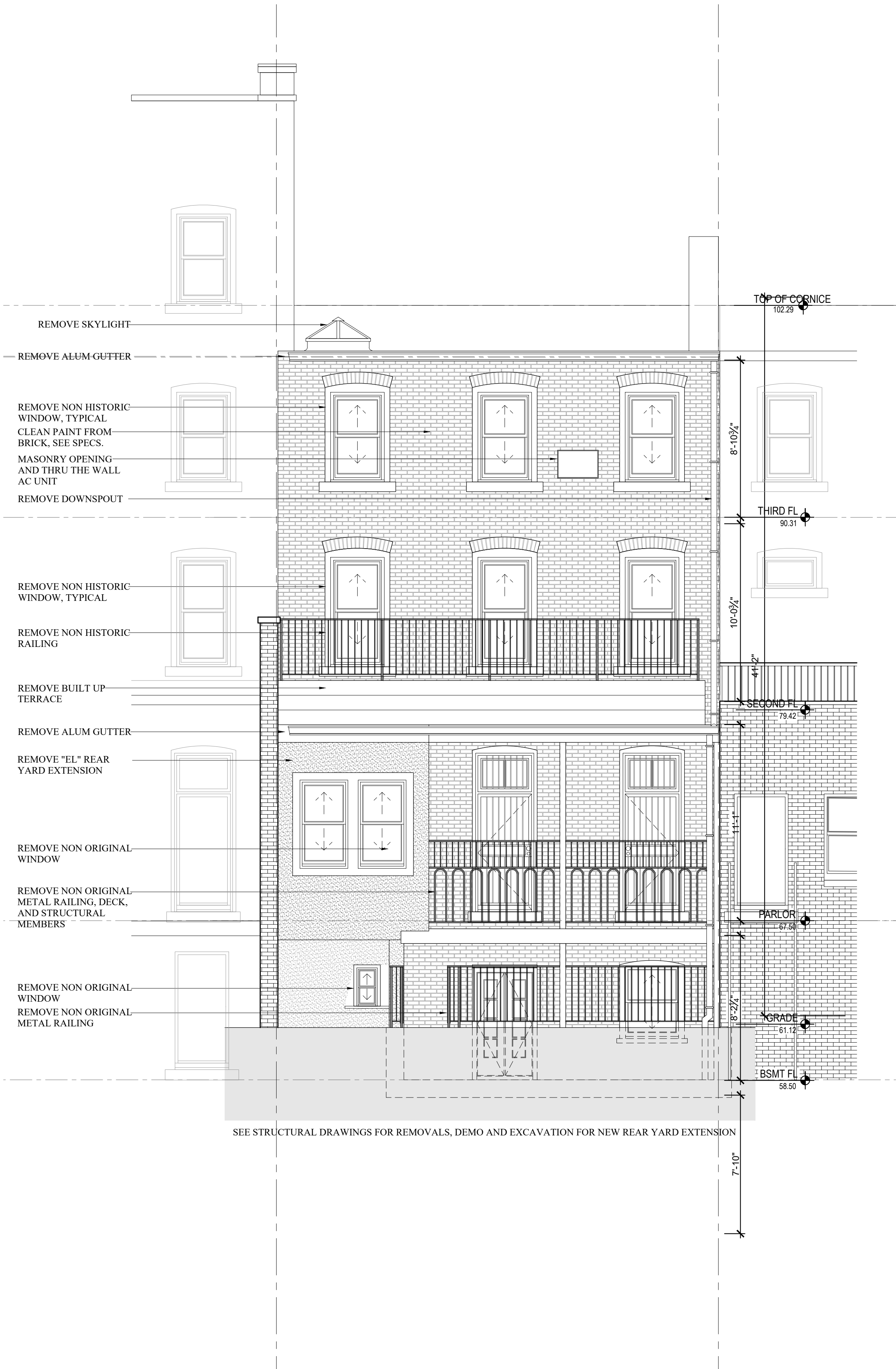
1 EXISTING CONDITION REAR ELEVATION 3/8" = 1'-0"
