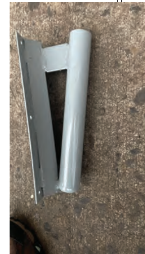
PAINTED STEEL PLATE- 9.5" H X 3.25" W DEPTH TOP: 4.5" 6 HOLES PAINTED BLACK TO MATCH AWNING PIPES
