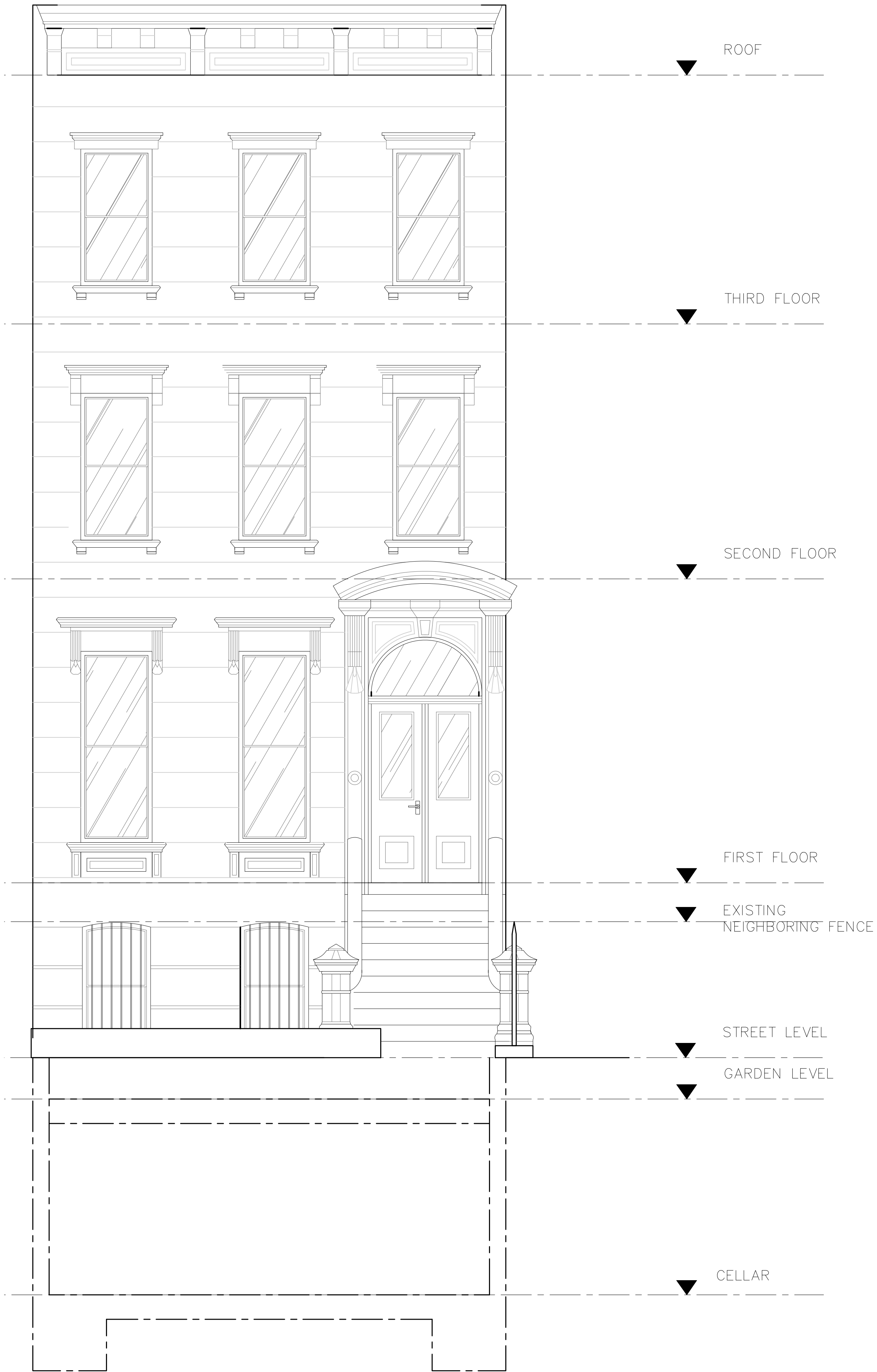
01 ELEVATION NORTH EXISTING CONDITION SCALE: 1/4" = 1'-0"
