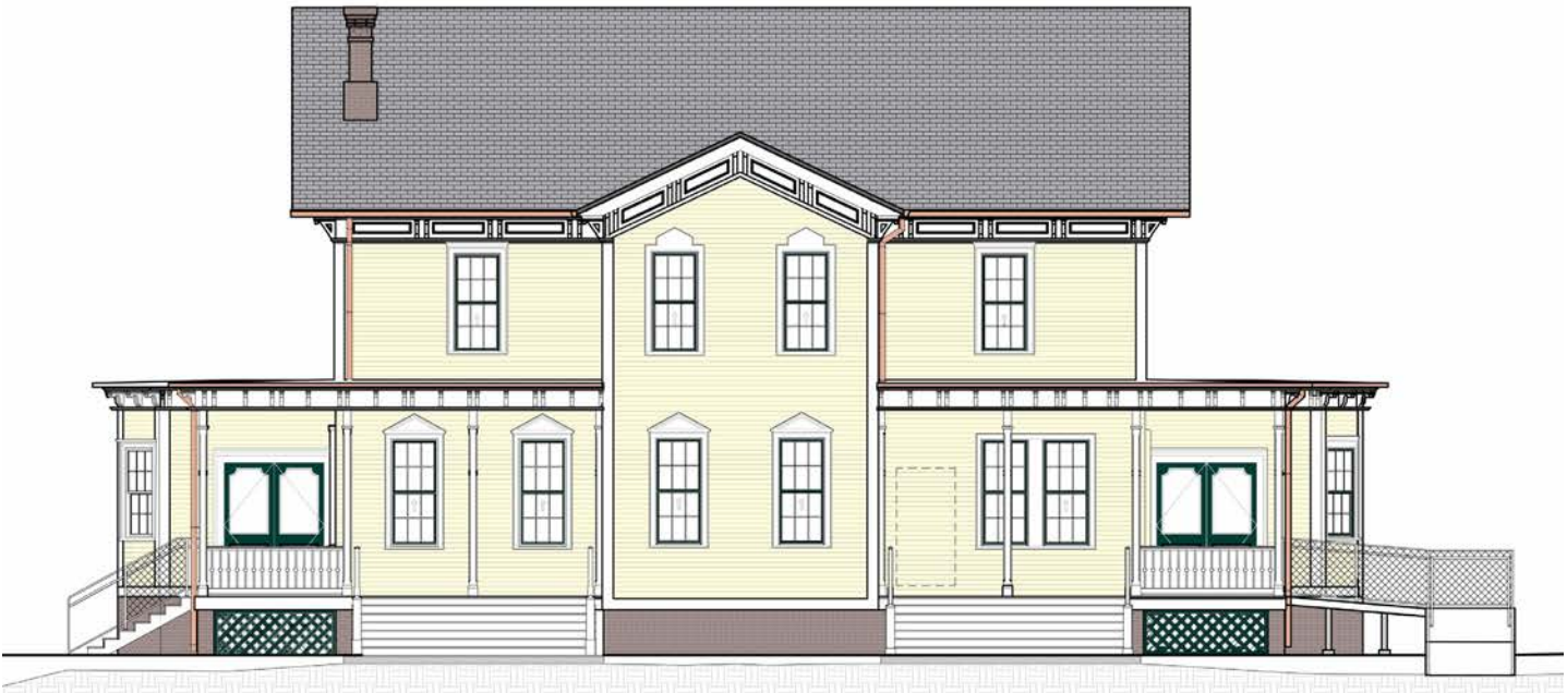
WOOD TRIMS, EAVES, COLUMNS, RAILING, WINDOWS & DOOR CASINGS Match Existing
