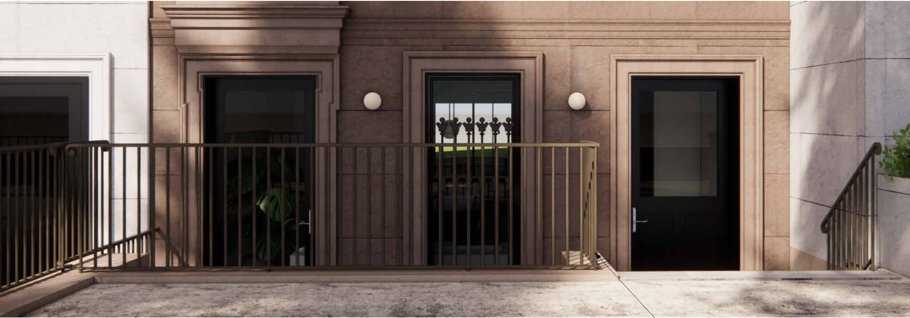
PROPOSED FRONT YARD - GUARDRAILS TO BE REUSED AND/OR REPLICATED TO MATCH EXISTING
