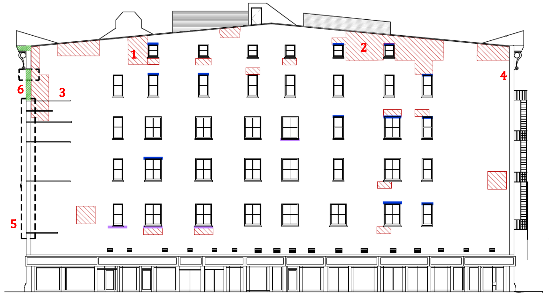
East Façade (Church St) - Existing Conditions
