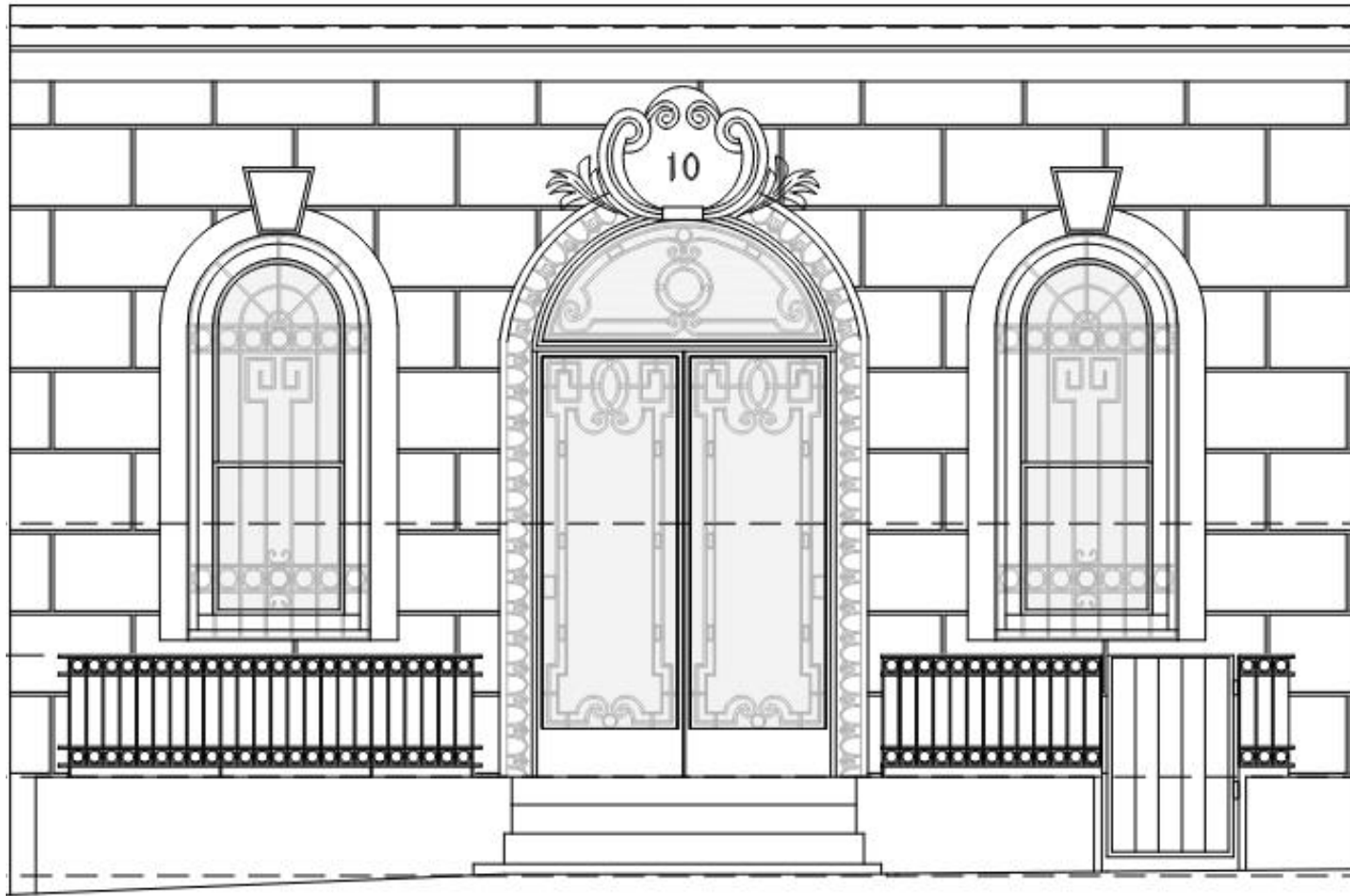
Existing Areaway Railing
