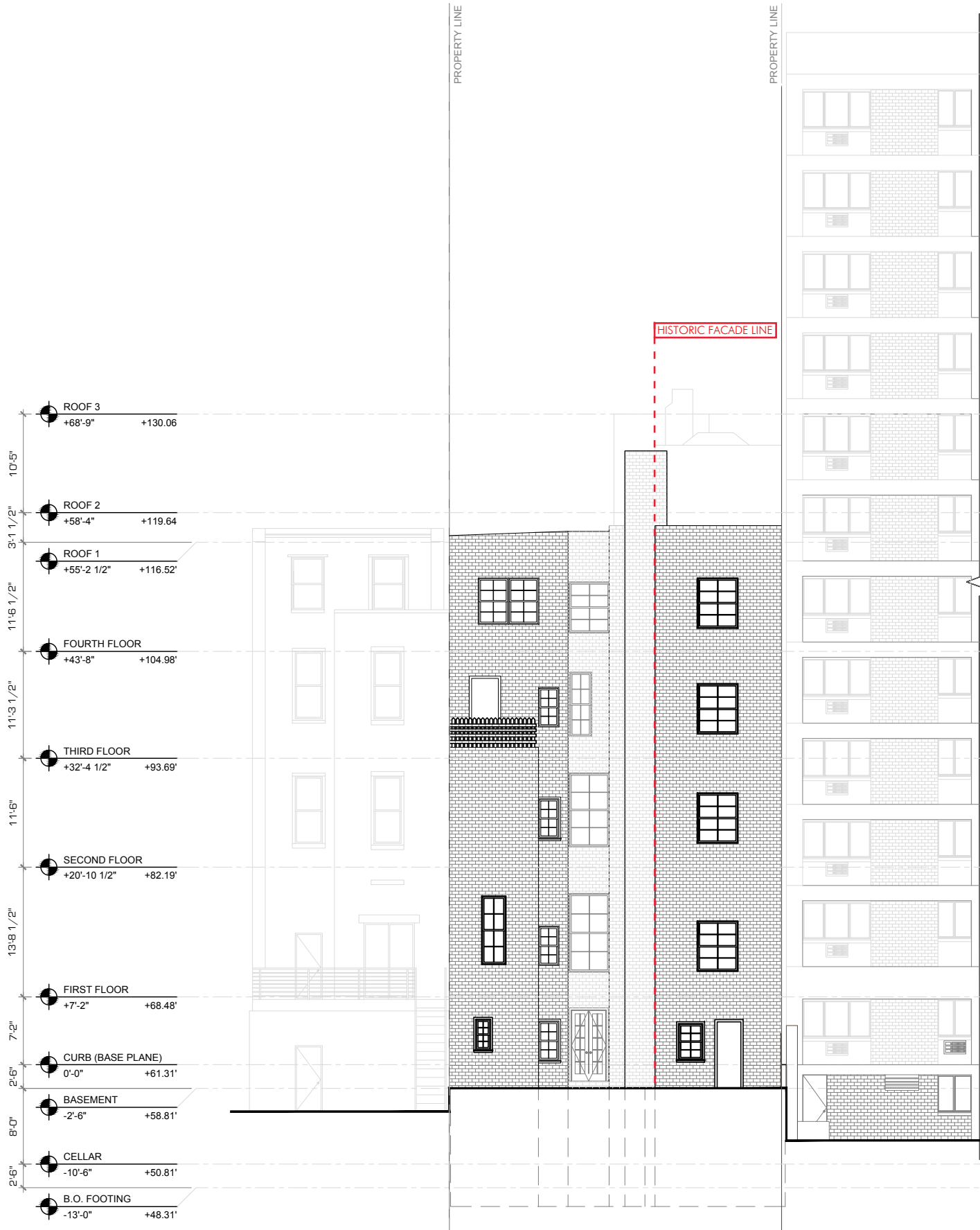
1 EXISTING EXTERIOR ELEVATION - REAR SCALE: 1/8" = 1'-0"
