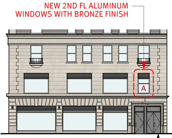
PROPOSED NORTH ELEVATION at E70th St.
