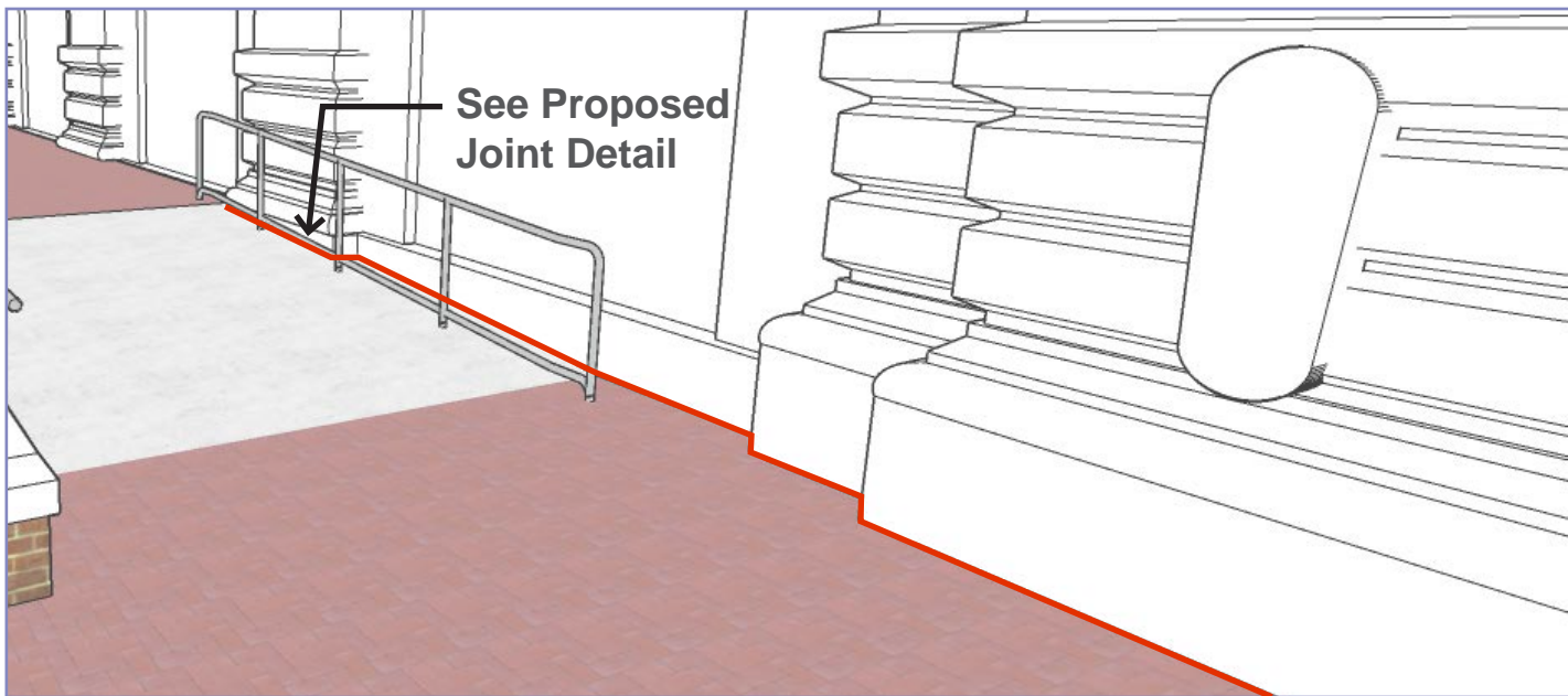
2 - Proposed Concrete Ramp at North Stair
