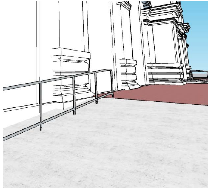
Replacement Stainless Steel Handrails
