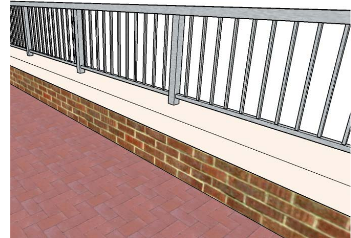
Replacement Stainless Steel Guardrail on Parapet
