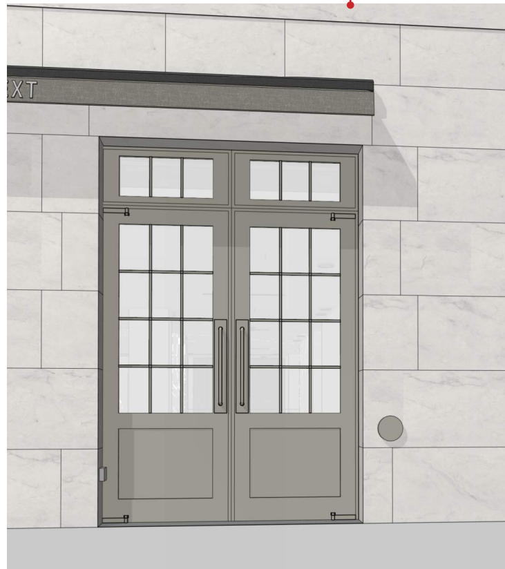
PROPOSED BALANCED PAINTED METAL & GLASS DOUBLE DOORS WITH 1/4" RECESSED LOWER PANELS AT EXTENDED MASONRY OPENING
