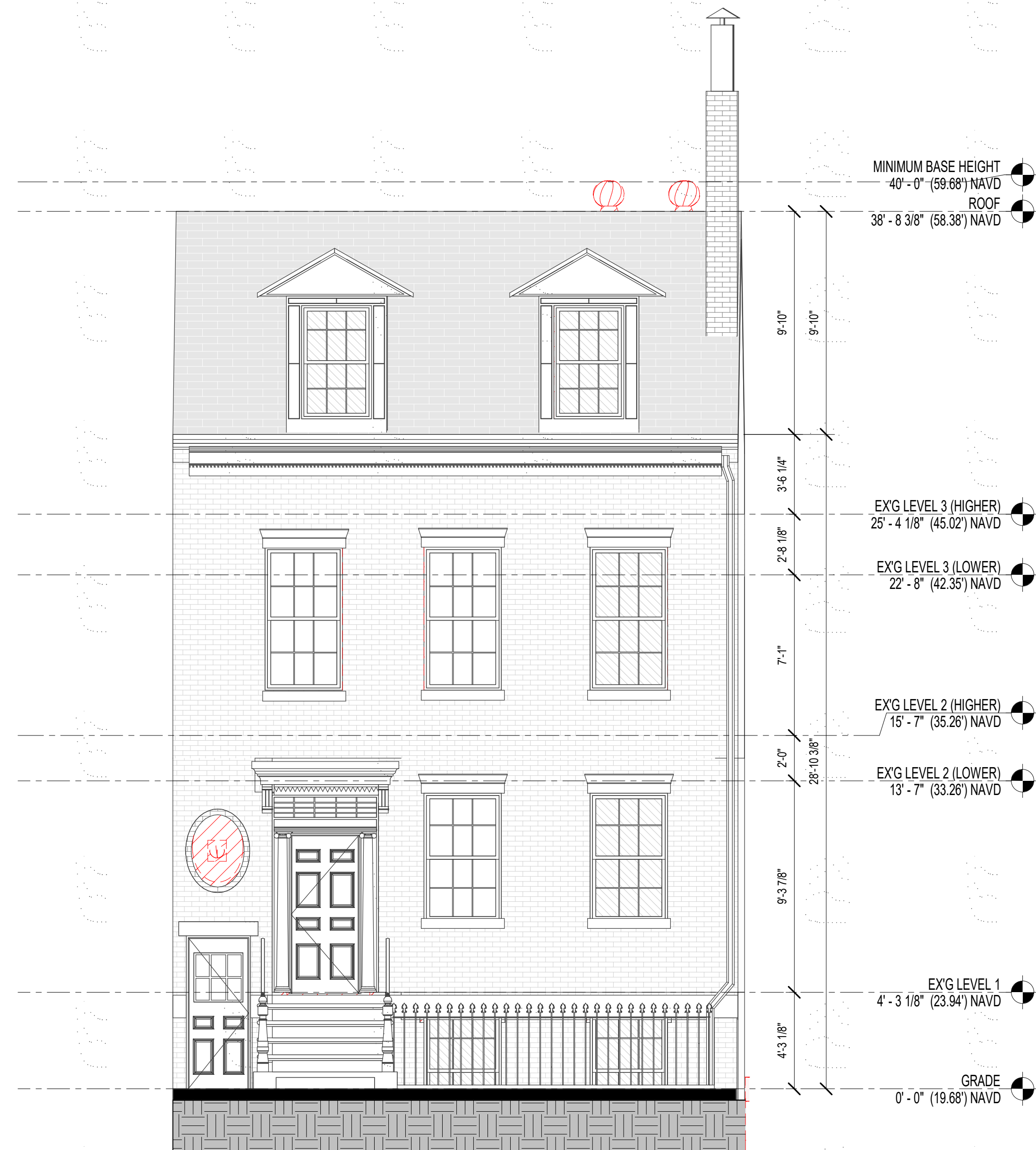
EXISTING ELEVATION - FRONT
