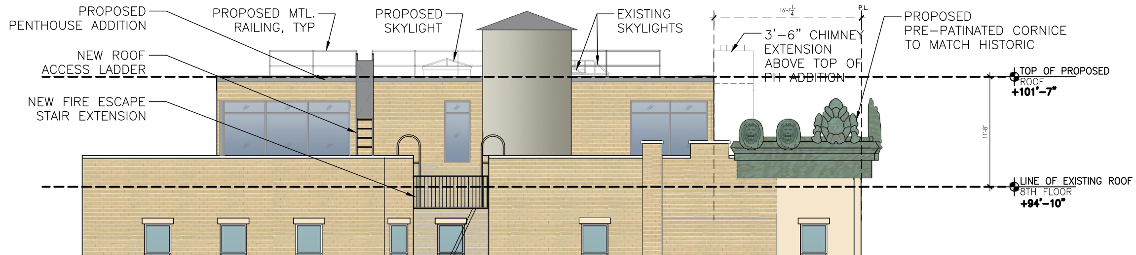
PROPOSED ELEVATION ANNEX ELEVATION - EAST
