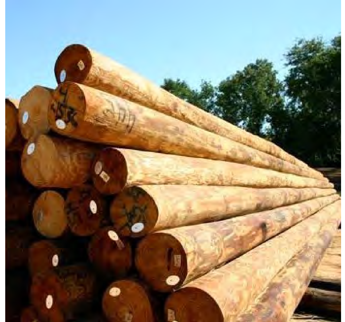
Southern Yellow Pine is the most common, durable utility pole material available.
