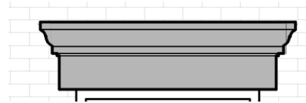
NEW LINTEL DETAIL-TYP.
