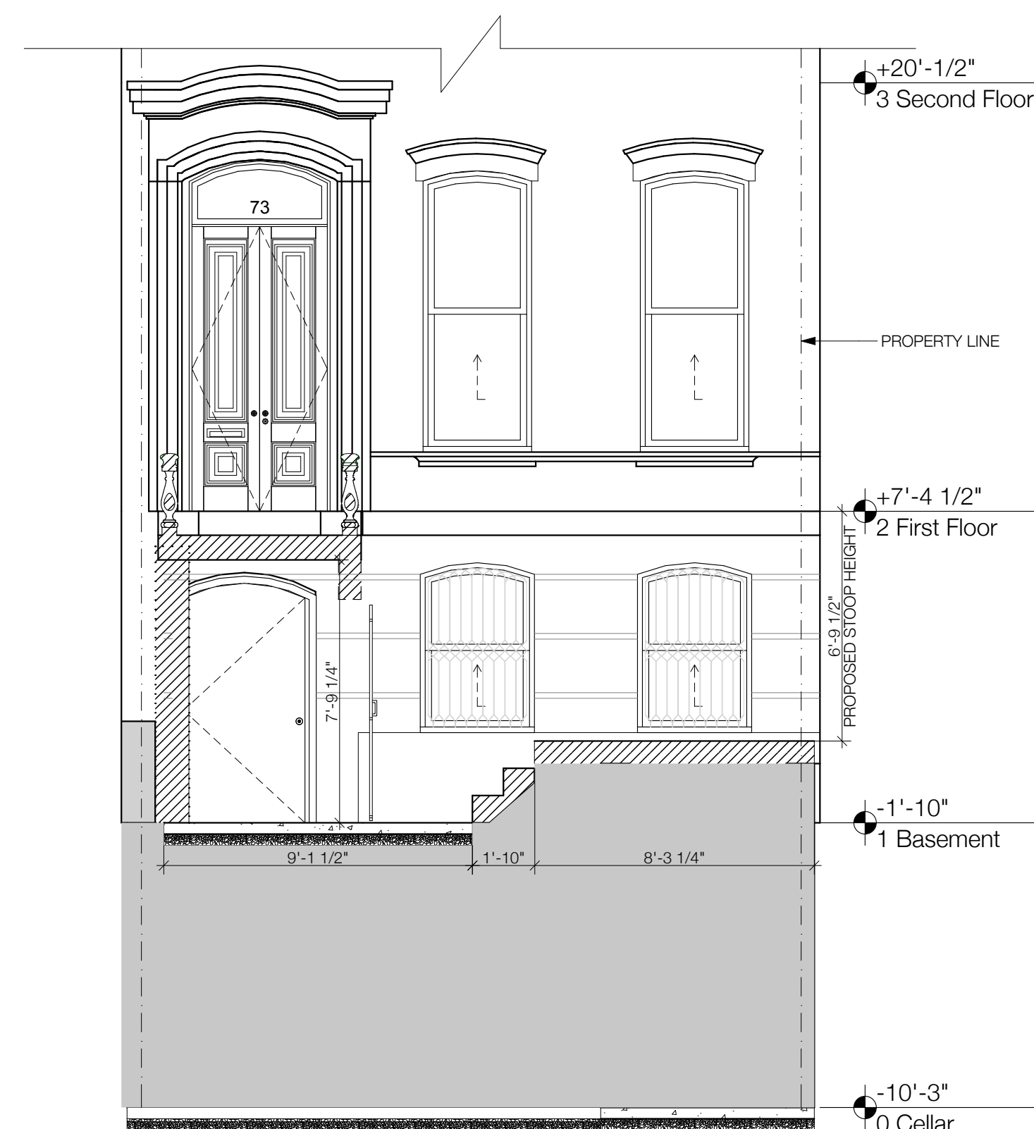
3 Proposed Basement Areaway Section SCALE: 1/4" = 1'-0"
