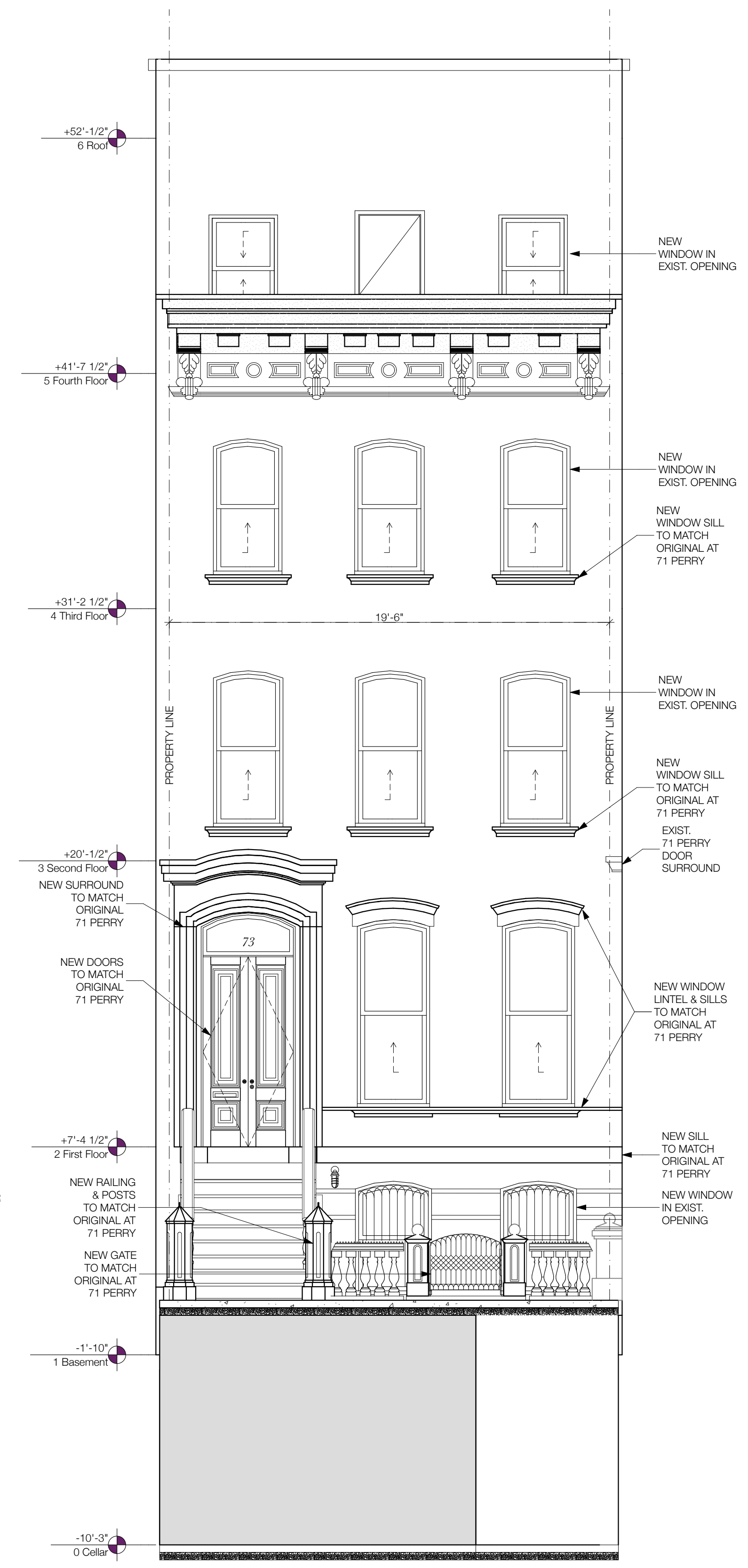
1 Proposed Front Elevation SCALE: 1/4" = 1'-0"
