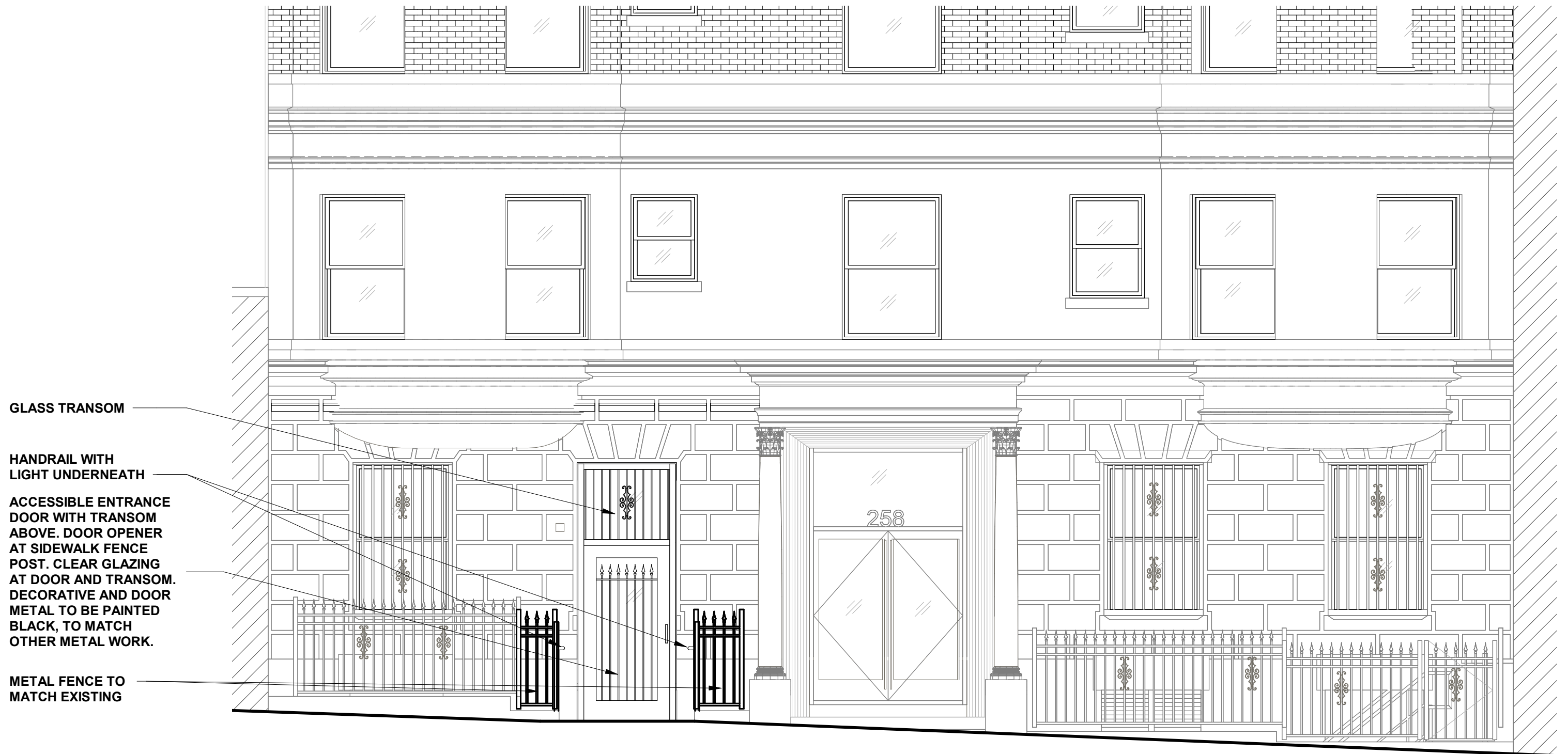
1 ENLARGED NORTH (FRONT) FACADE LPC-09 1/4" = 1'-0"
