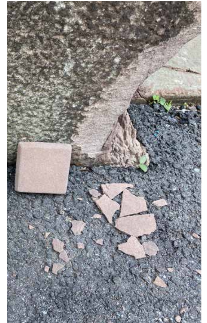
'Fiske 18' Cast stone, as pictured in front of original Portland brownstone pier.
