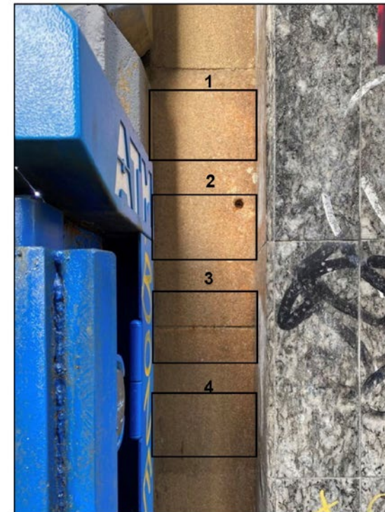
Figure 5. Test Area 2 After: 1) Prosoce Sure Klean Heavy Duty Paint Stripper, 24 hour dwell, 2) Dumond Smart Strip, 24 hour dwell, 3) Prosoce Enviro Klean Safstrip 8, 24 hour dwell, 4) Back to Nature Multistrip, 24 hour dwell, 5) Dumond Peel Away 1, 24 hour dwell, 6) Dumond Smart Strip Pro, 24 hour dwell, 7) Shorebest SB2220, 30 minute dwell, 8) Shorebest SB2230, 15 minute dwell
