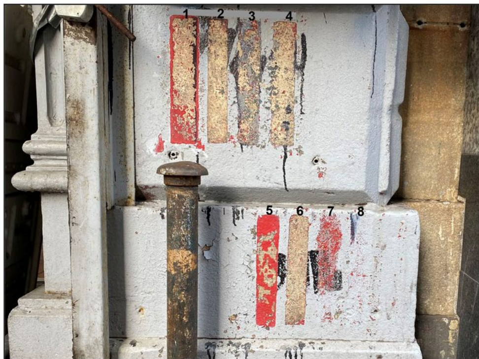
Figure 3. Test Area 1 After: 1) Prosoce Sure Klean Heavy Duty Paint Stripper, 24 hour dwell, 2) Dumond Smart Strip, 24 hour dwell, 3) Prosoce Enviro Klean Safstrip 8, 24 hour dwell, 4) Back to Nature Multistrip, 24 hour dwell, 5) Dumond Peel Away 1, 24 hour dwell, 6) Dumond Smart Strip Pro, 24 hour dwell, 7) Shorebest SB2220, 30 minute dwell, 8) Shorebest SB2230, 15 minute dwell
